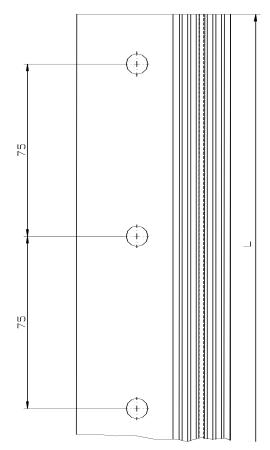
Vertical connection profile - "villerit Verbindungsschiene" (dimensions in millimetres)
