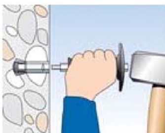
4.) Drive in the pin with the setting tool
