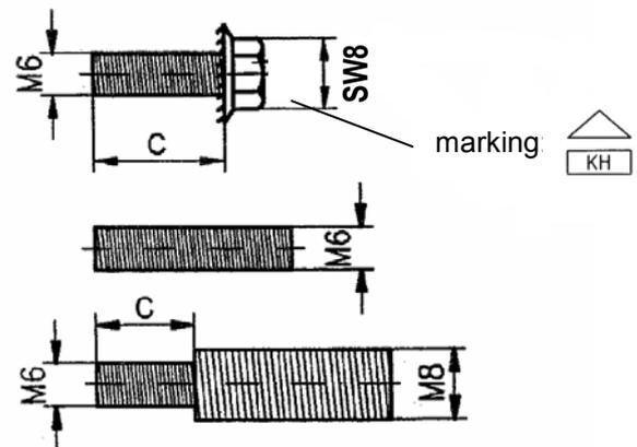
c: the length of the thread has to be adapted to the respective substructure and setting depth of the anchor
