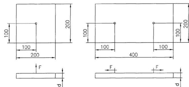
**Figure 6:** tension test or shear test for an edge distance 100 / 100 mm
