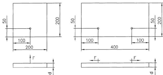
**Figure 5:** tension test or shear test for an edge distance 50 / 100 mm
