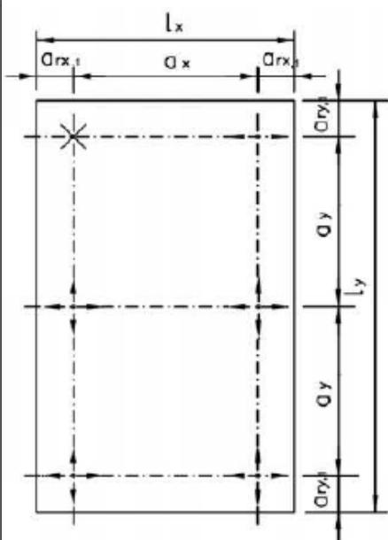
**Figure 13:** Façade panel with 6 agraffes – support condition 2
