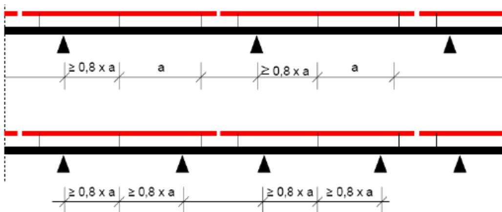
**Figure 10:** In profiles, supporting three fixing points of a panel, the central fixing points must have a minimum distance of  $0,8 \times a$  ( $a$ = spacing of the fixing points of the panel) to the supports.
