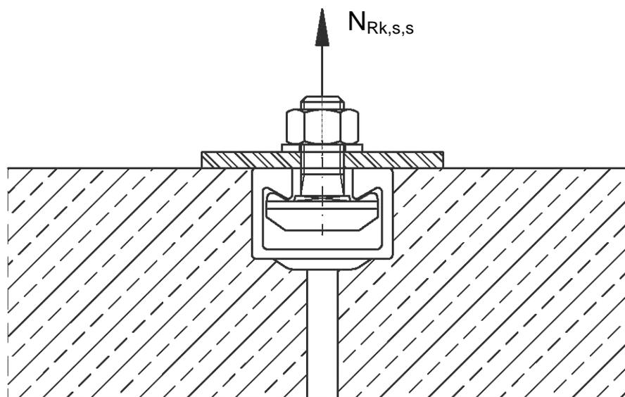
Channel under tension load
