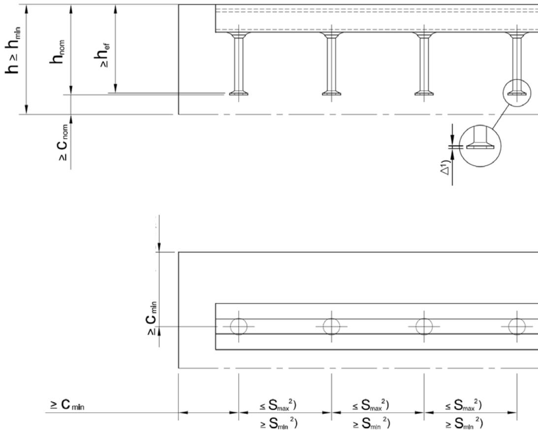
Table 9: Minimum anchorage depth, edge distance and member thickness for cold rolled profiles
