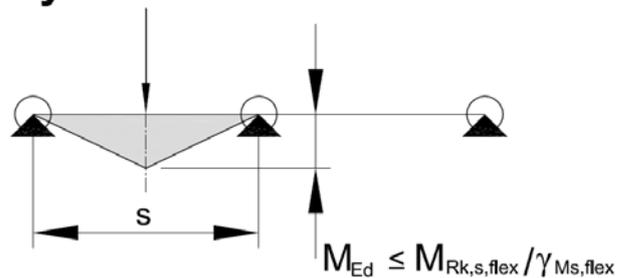
Table 13: Flexure resistance of channel
