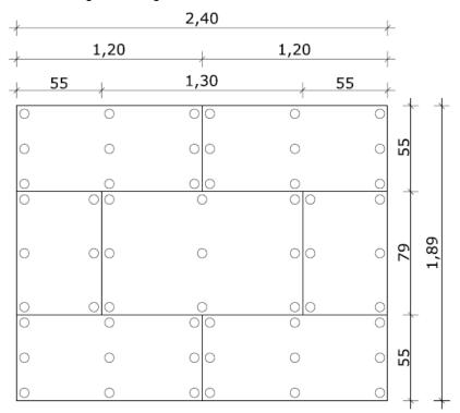
The following anchoring scheme shall be used with insulation thickness more than 100 mm (in two layers):
