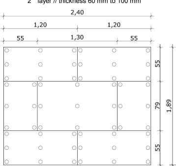
2<sup>nd</sup> layer // thickness 60 mm to 100 mm
