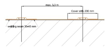
Maximum distance between lines of point fixation: ≤ 1,88 m
