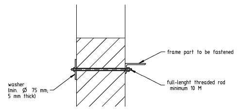
type 2 concrete walls, min. 200 mm thick dowels according to control plan of 11 January 2012
