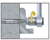
4. Apply the required installation torque T<sub>inst</sub> by using a torque wrench
