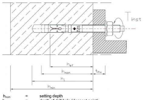
depth of drill hole (deepest point) h<sub>1</sub> min. thickness of concrete member hmin
