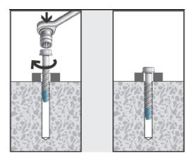
Placing the fixture and setting the screw
