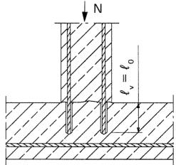
Note to Figure 1 to 5: In the figures no transverse reinforcement is plotted, the transverse reinforcement as required by EN 1992-1-1 shall be present.
