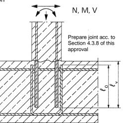
**Figure 4:** Rebar connection for components stressed primarily in compression. The rebars sre stressed in compression
