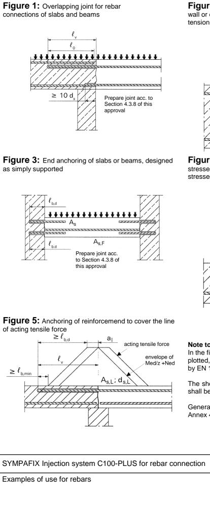
**Figure 2:** Overlapping joint at a foundation of a wall or column where the rebars are stressed in tension
