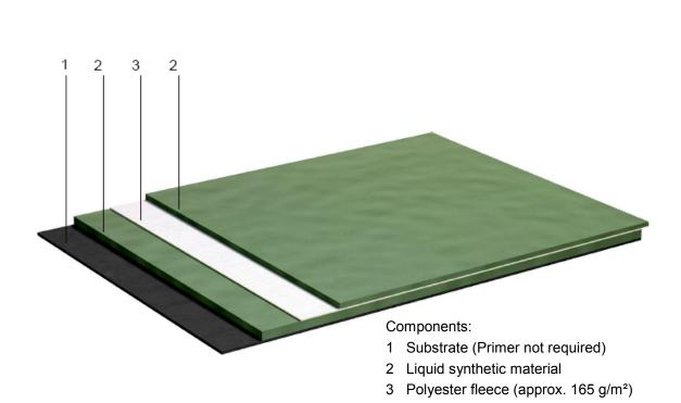
Applicable to the roof waterproofing system "StoPma Waterproofing System":
