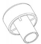
Piston plug for overhead or horizontal installation  $All\ diameter\ (d_0)$
