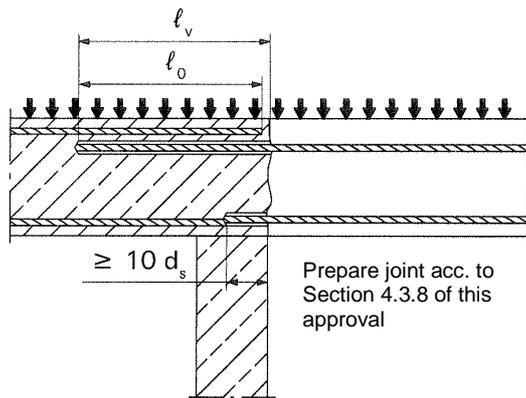
**Figure 2:** Overlapping joint at a foundation of a wall or column where the rebars are stressed in tension
