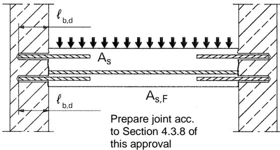
**Figure 4:** Rebar connection for components stressed primarily in compression. The rebars are stressed in compression
