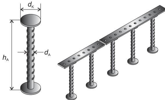
**Figure 1: Double headed stud with steel rails welded to the heads**
