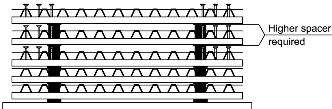
When storing and transporting precast elements, the height of the HDB Double-Headed Stud-Elements has to be considered. Higher spacers are required when stacking the precast elements.
