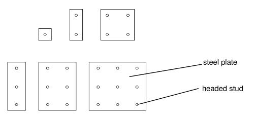
Other arrangements e.g. in a triangular or circular pattern are also allowed; however, the provisions of this design method should be applied with engineering judgement.
