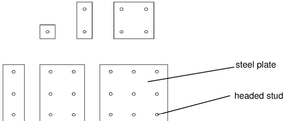
Other arrangements e.g. in a triangular or circular pattern are also allowed; however, the provisions of this design method should be applied with engineering judgement.
