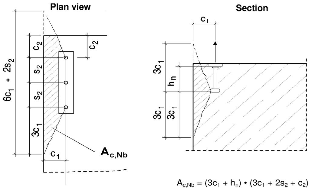
**Figure 4 :** Idealized concrete cone of the headed stud in the case of local concrete blow-out failure at the edge
