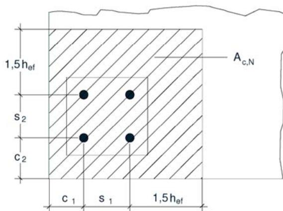
$$A_{c,N} = (c_1 + s_1 + 1.5h_{ef}) \cdot (c_2 + s_2 + 1.5h_{ef})$$
