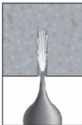
Blow out dust and fragments
