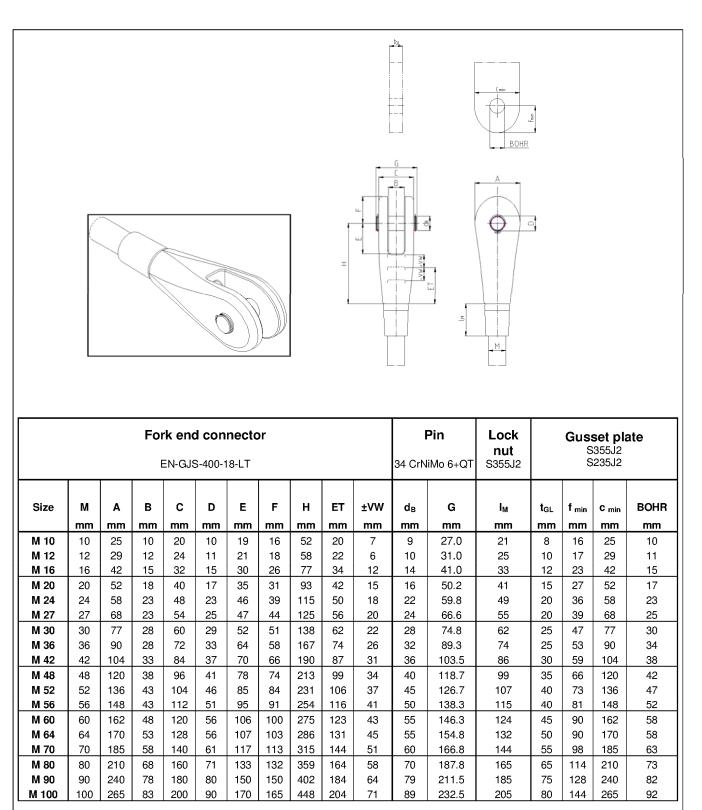
Fork end connector, pin, lock nut, gusset plate
