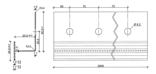
Vertical connection profile "Brillux WDVS Alu-Verbindungsleiste 3580" (dimensions in millimetres)
