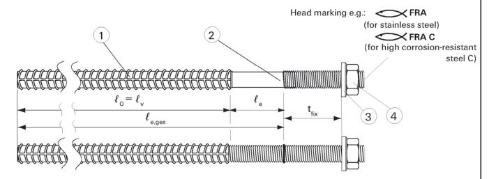
Table 1: Dimensions of rebar anchor FRA and FRA C
