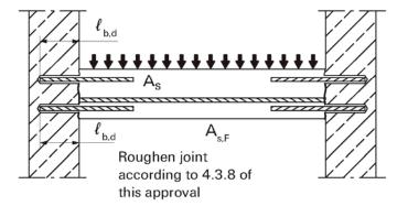
End anchoring of slabs or beams which have been designed as simply supported
