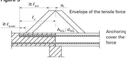
Anchoring of reinforcement to cover the envelope of the tensile force
