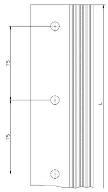
Vertical connection profile – "Duroflex PVC Verbindungsschiene" (dimensions in millimetres)
