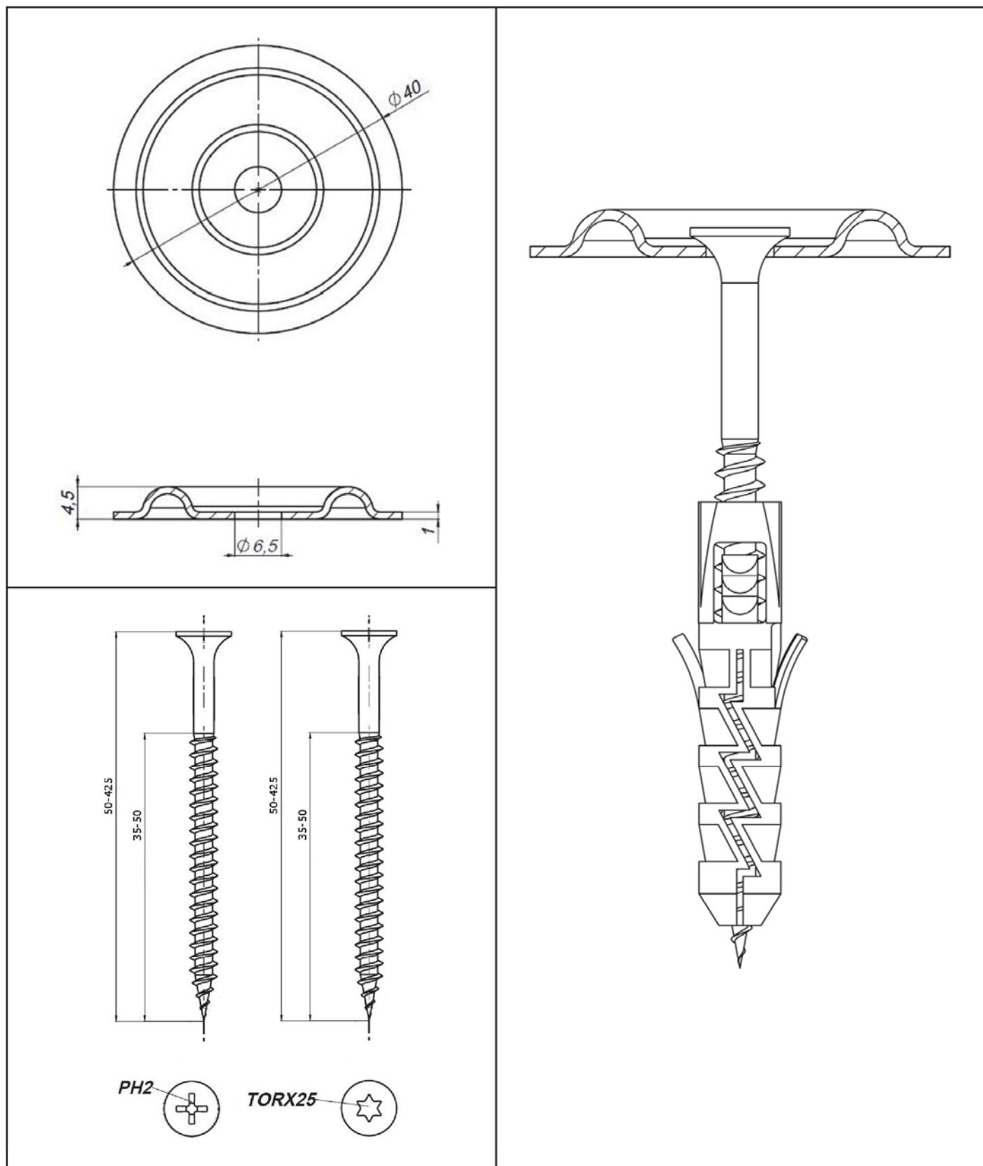
**KOELNER S.A. Flat Roof Fasteners**
