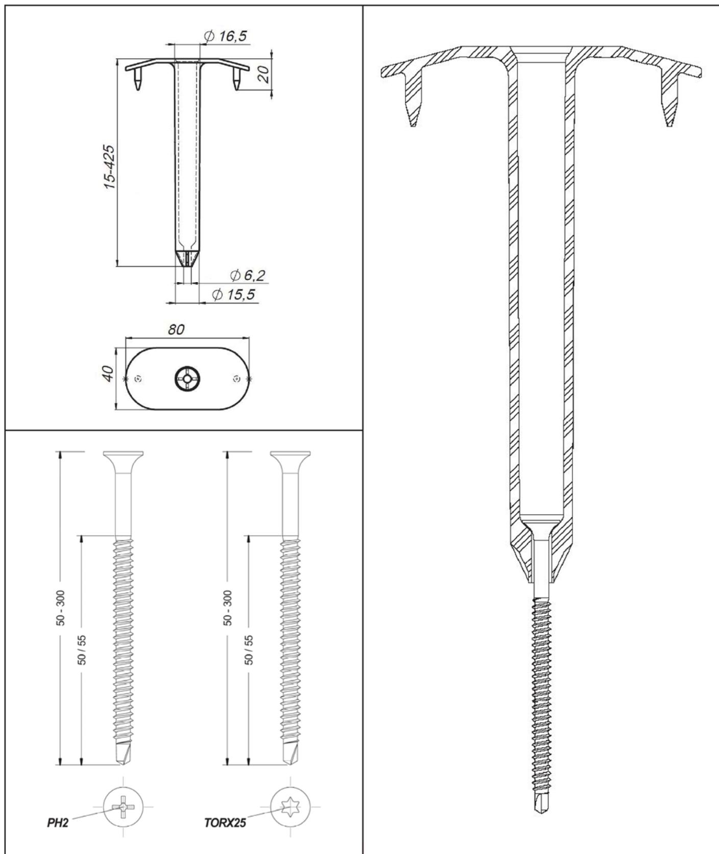
**KOELNER S.A. Flat Roof Fasteners**
