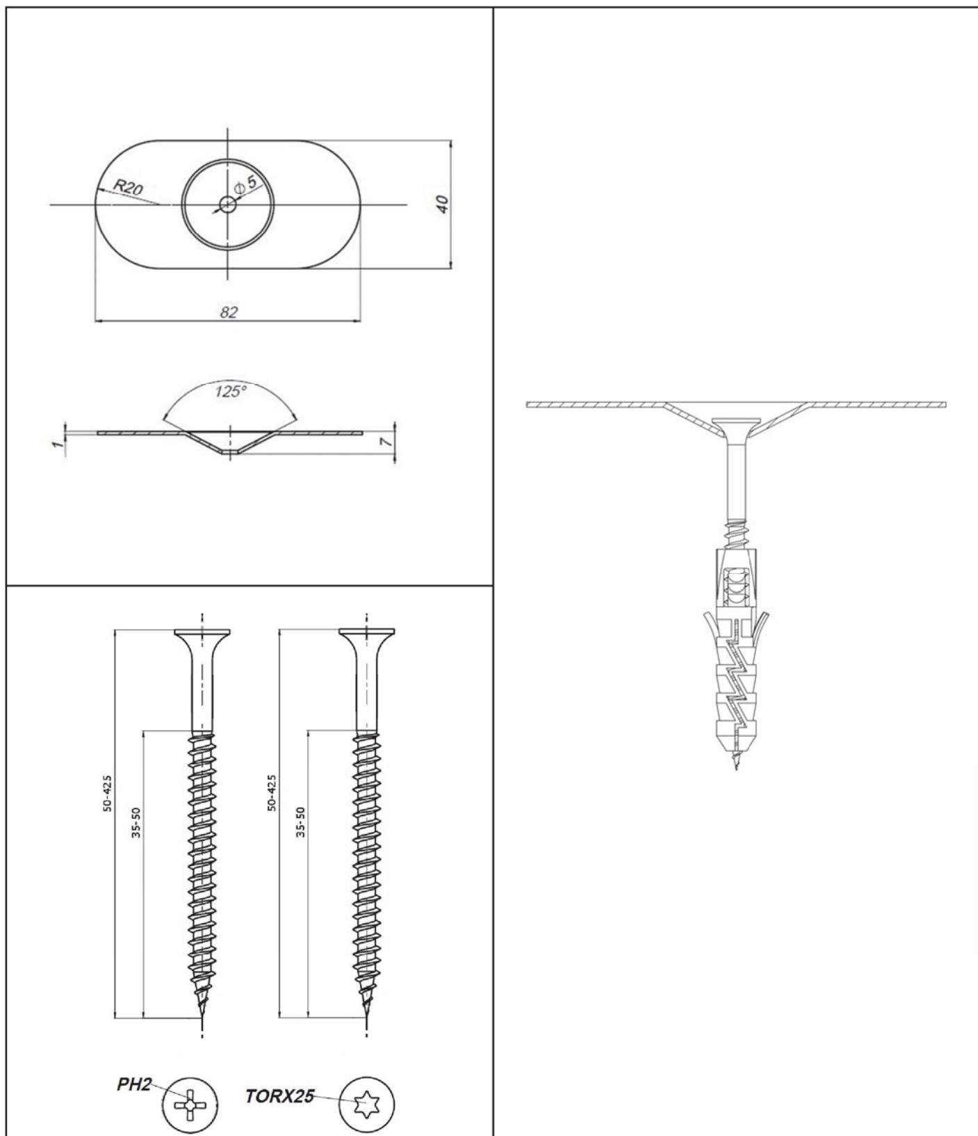
**KOELNER S.A. Flat Roof Fasteners**
