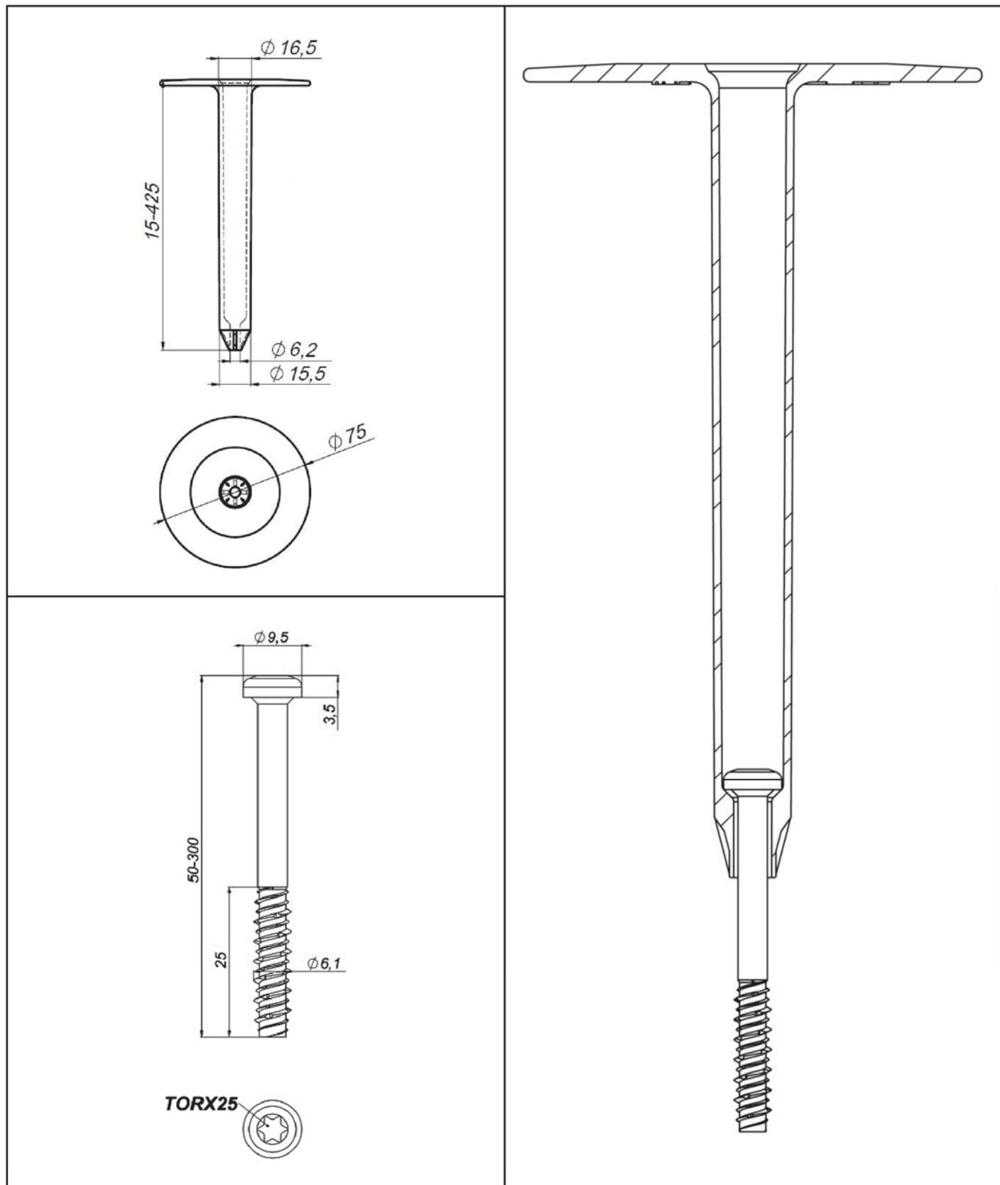
KOELNER S.A. Flat Roof Fasteners
