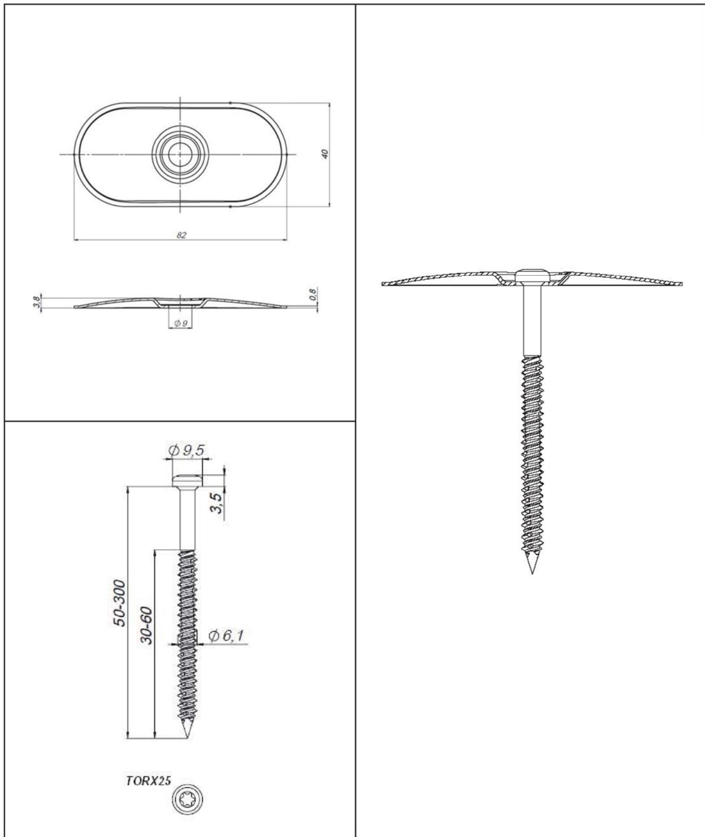
**KOELNER S.A. Flat Roof Fasteners**
