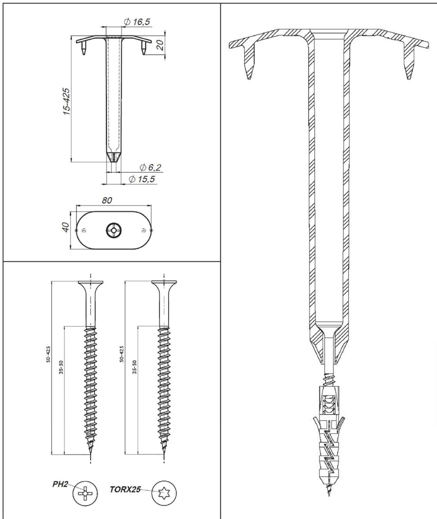
**KOELNER S.A. Flat Roof Fasteners**
