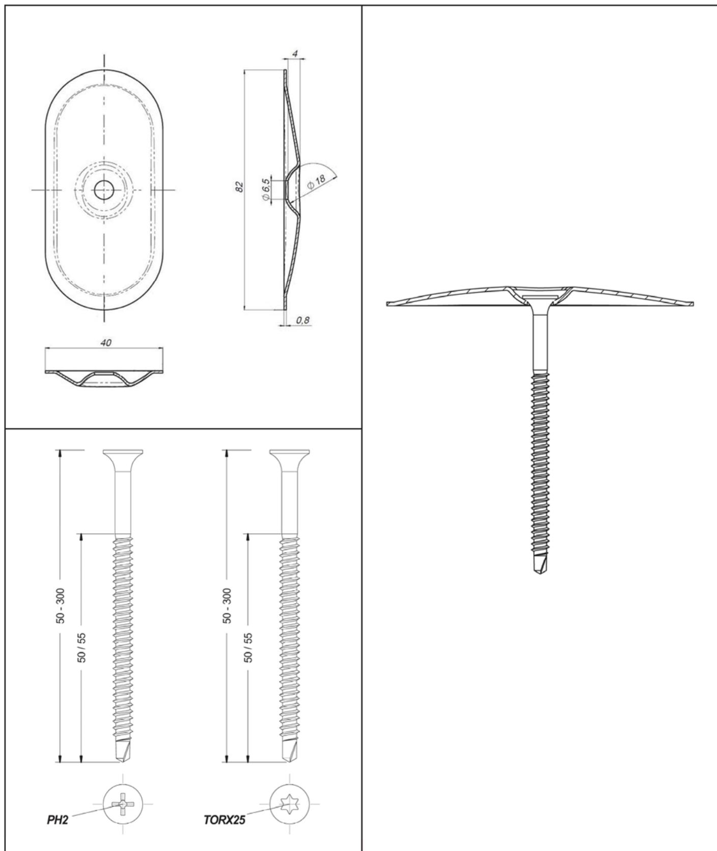
**KOELNER S.A. Flat Roof Fasteners**
