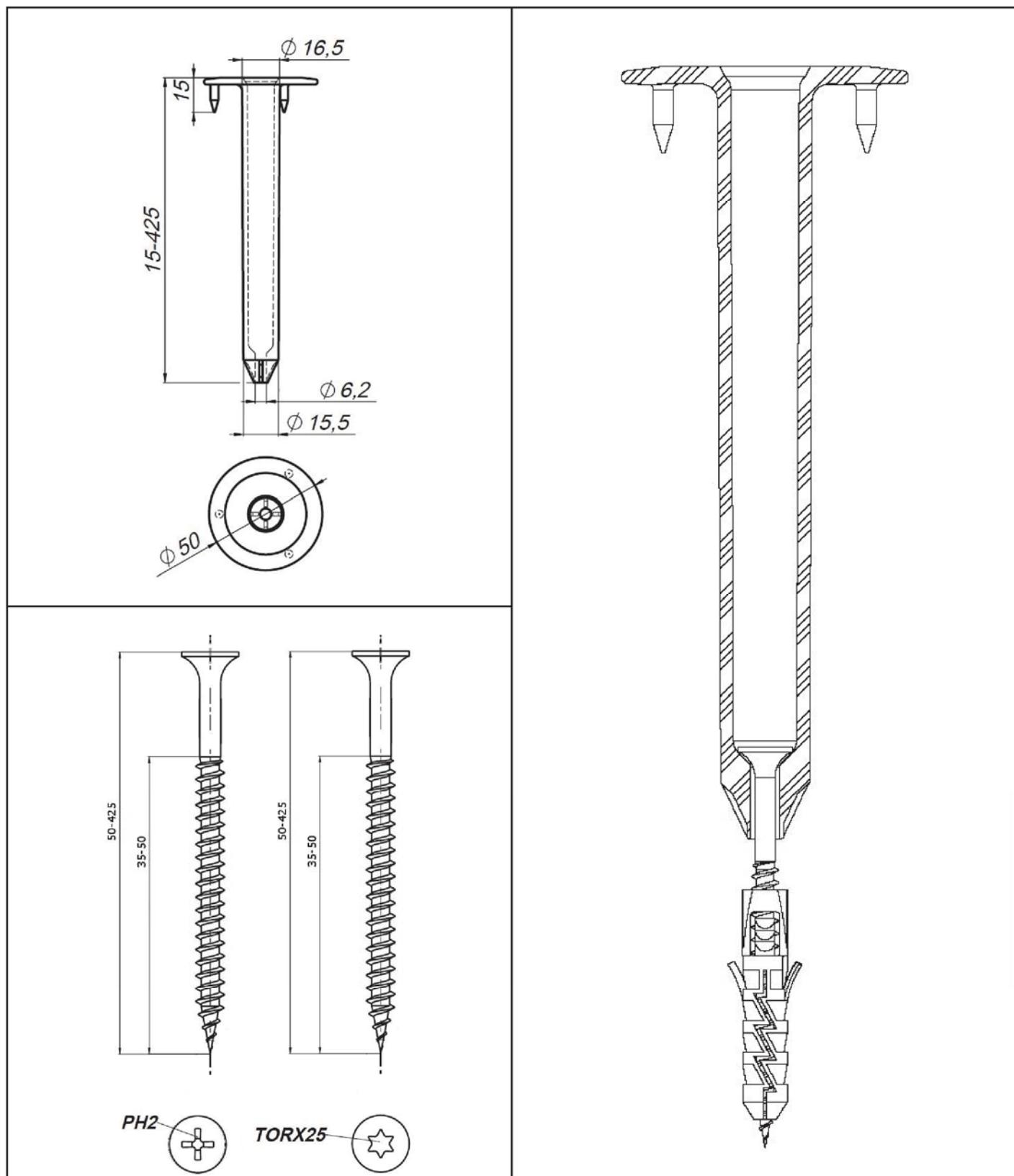
**KOELNER S.A. Flat Roof Fasteners**
