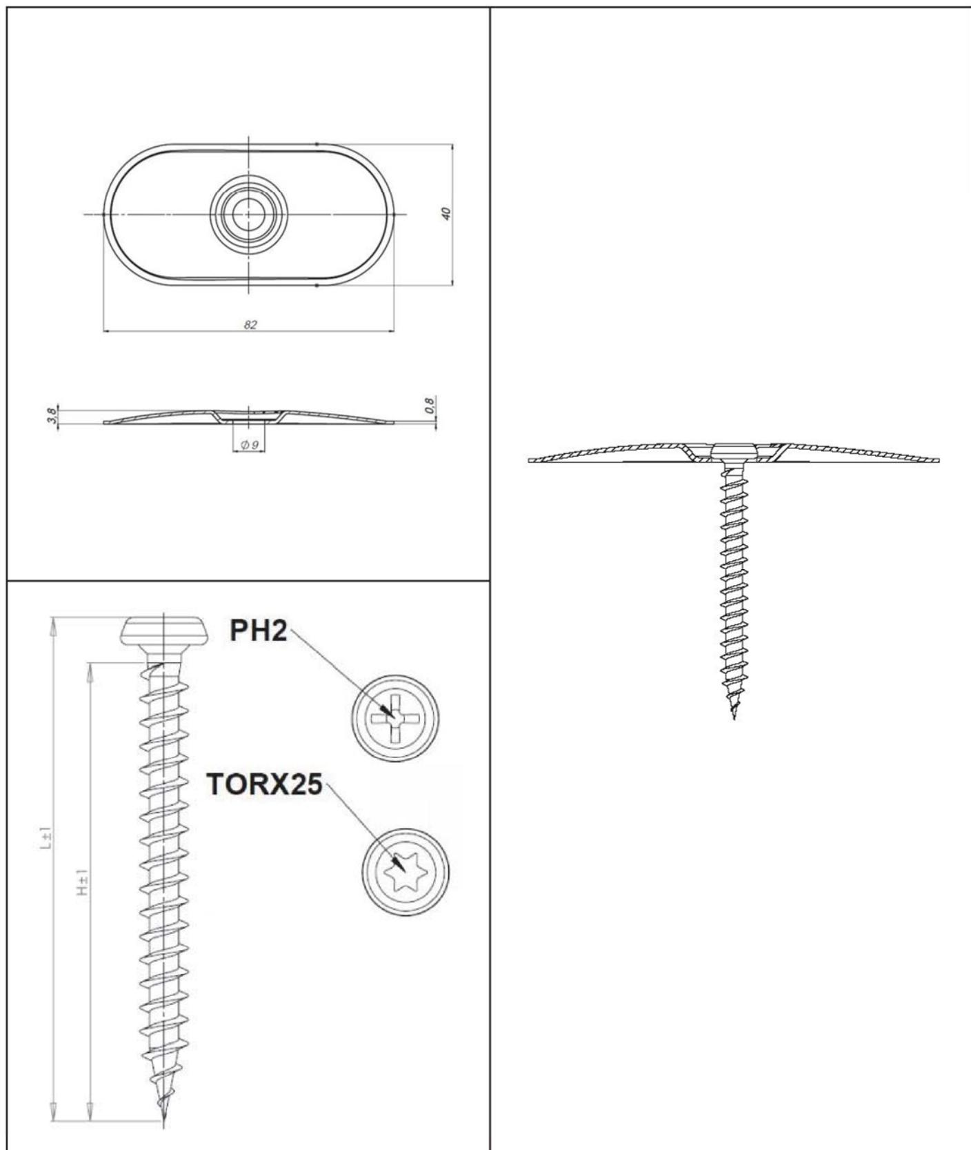
**KOELNER S.A. Flat Roof Fasteners**
