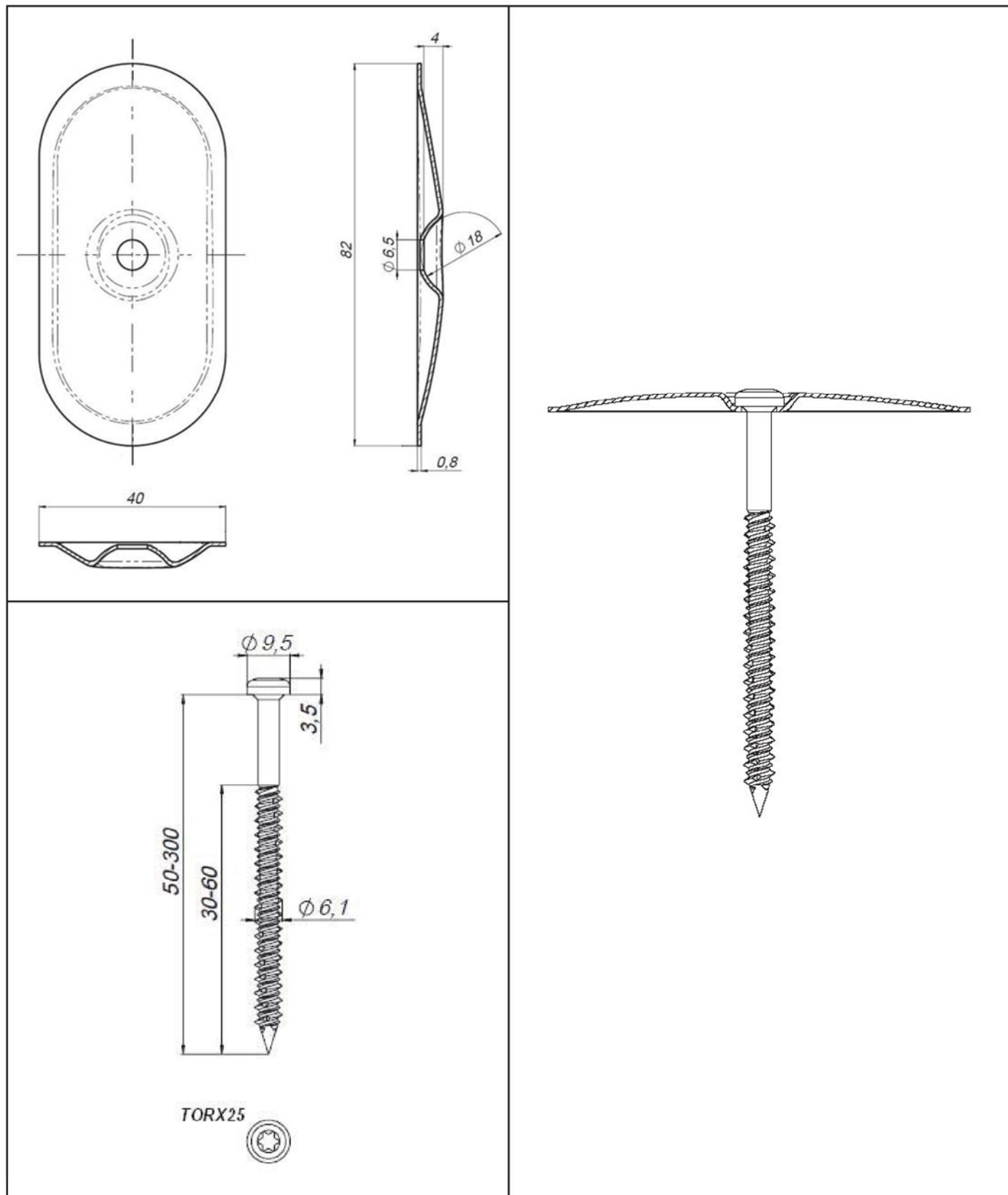
**KOELNER S.A. Flat Roof Fasteners**
