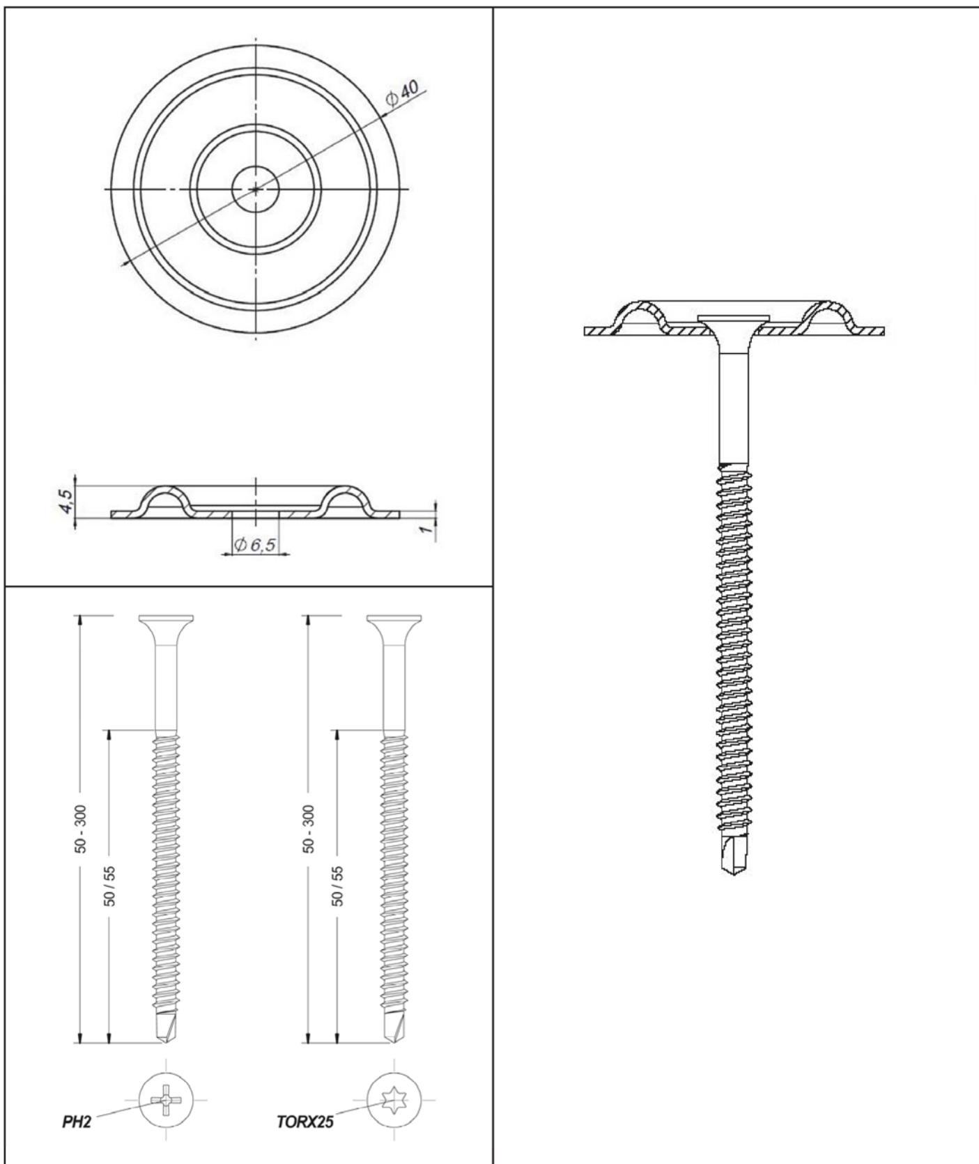
**KOELNER S.A. Flat Roof Fasteners**
