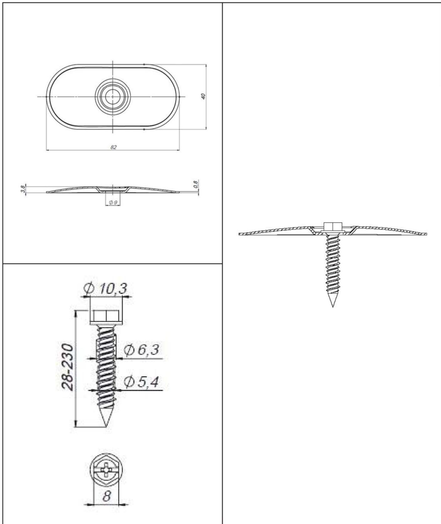
**KOELNER S.A. Flat Roof Fasteners**
