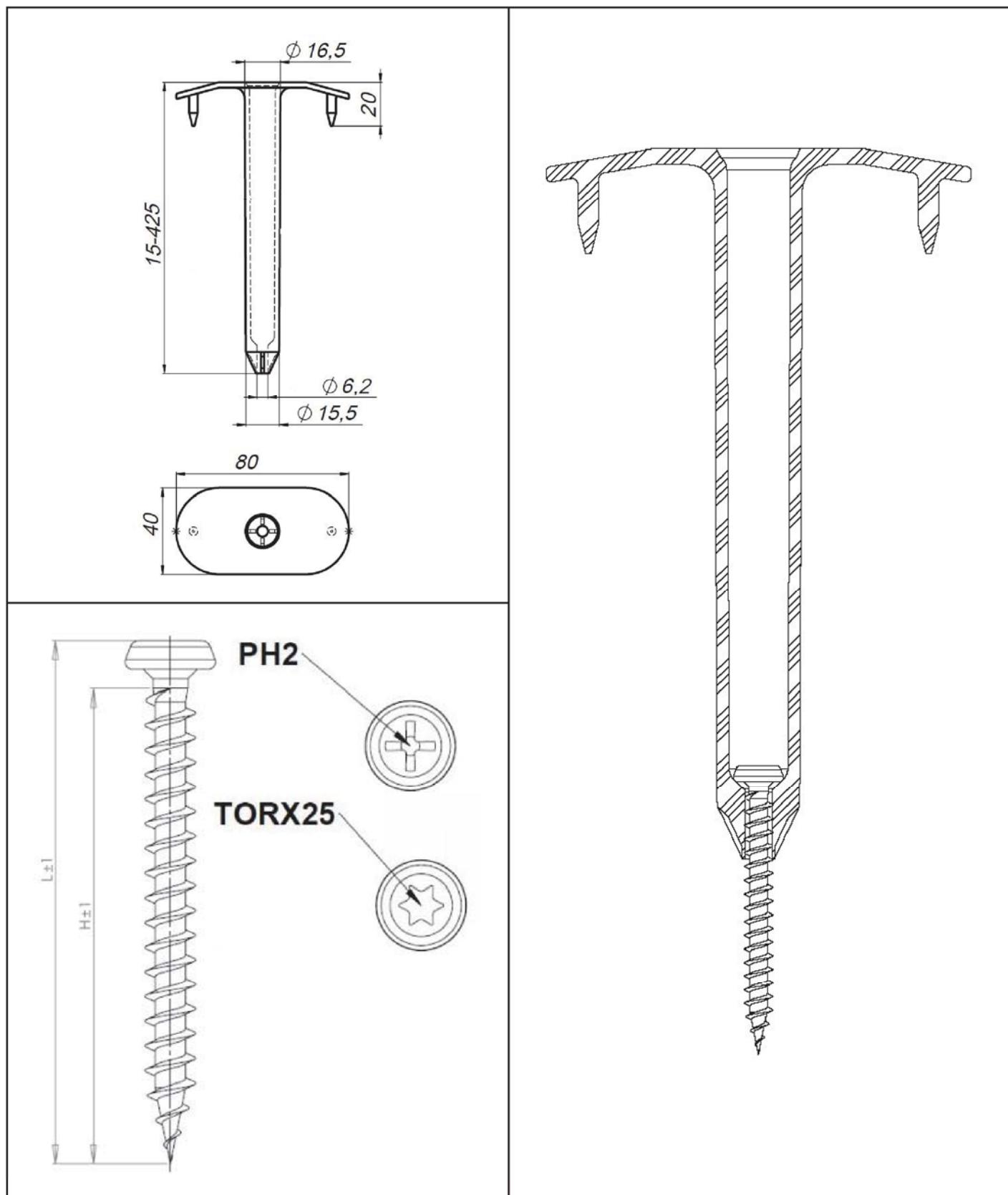
KOELNER S.A. Flat Roof Fasteners
