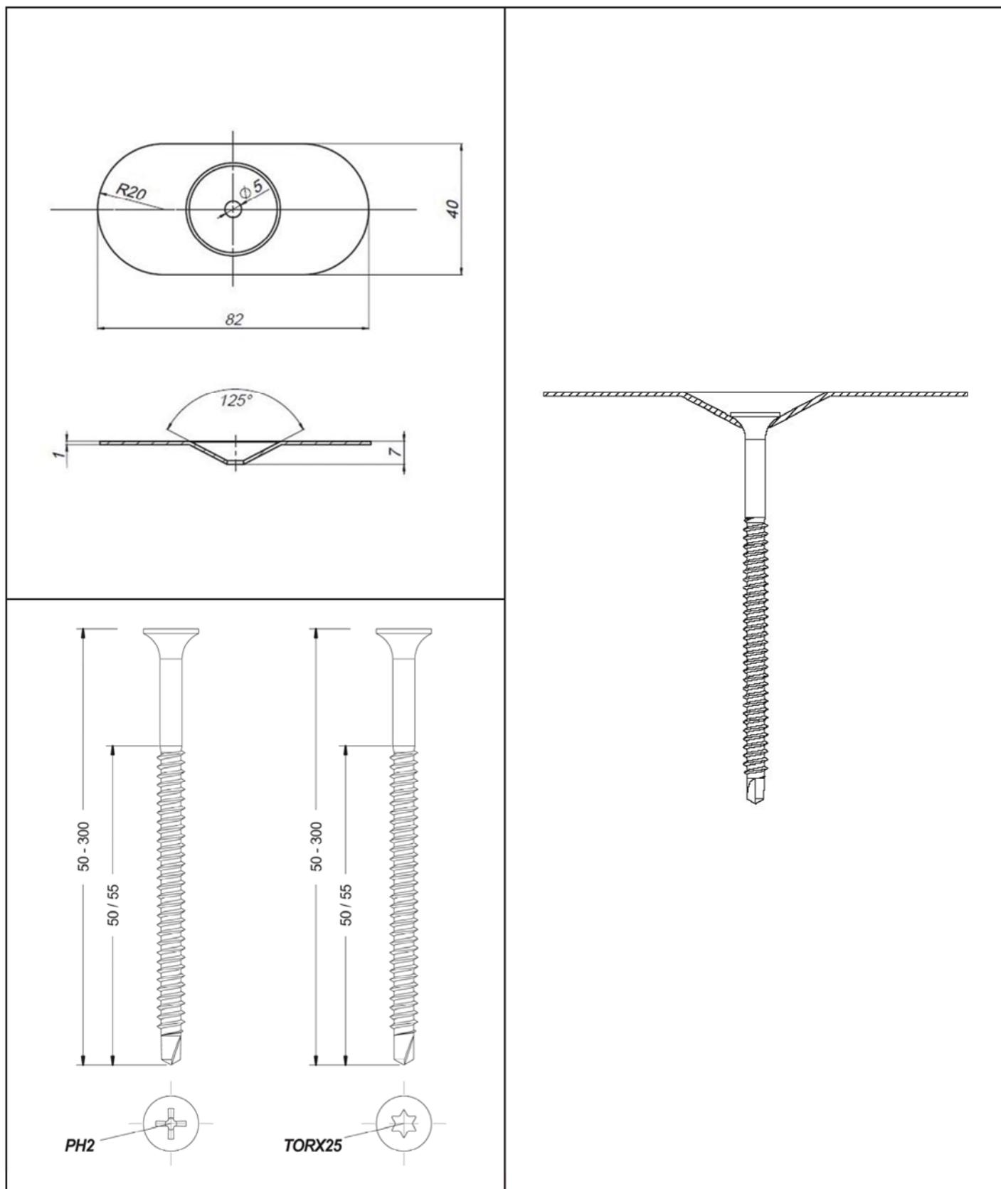
**KOELNER S.A. Flat Roof Fasteners**
