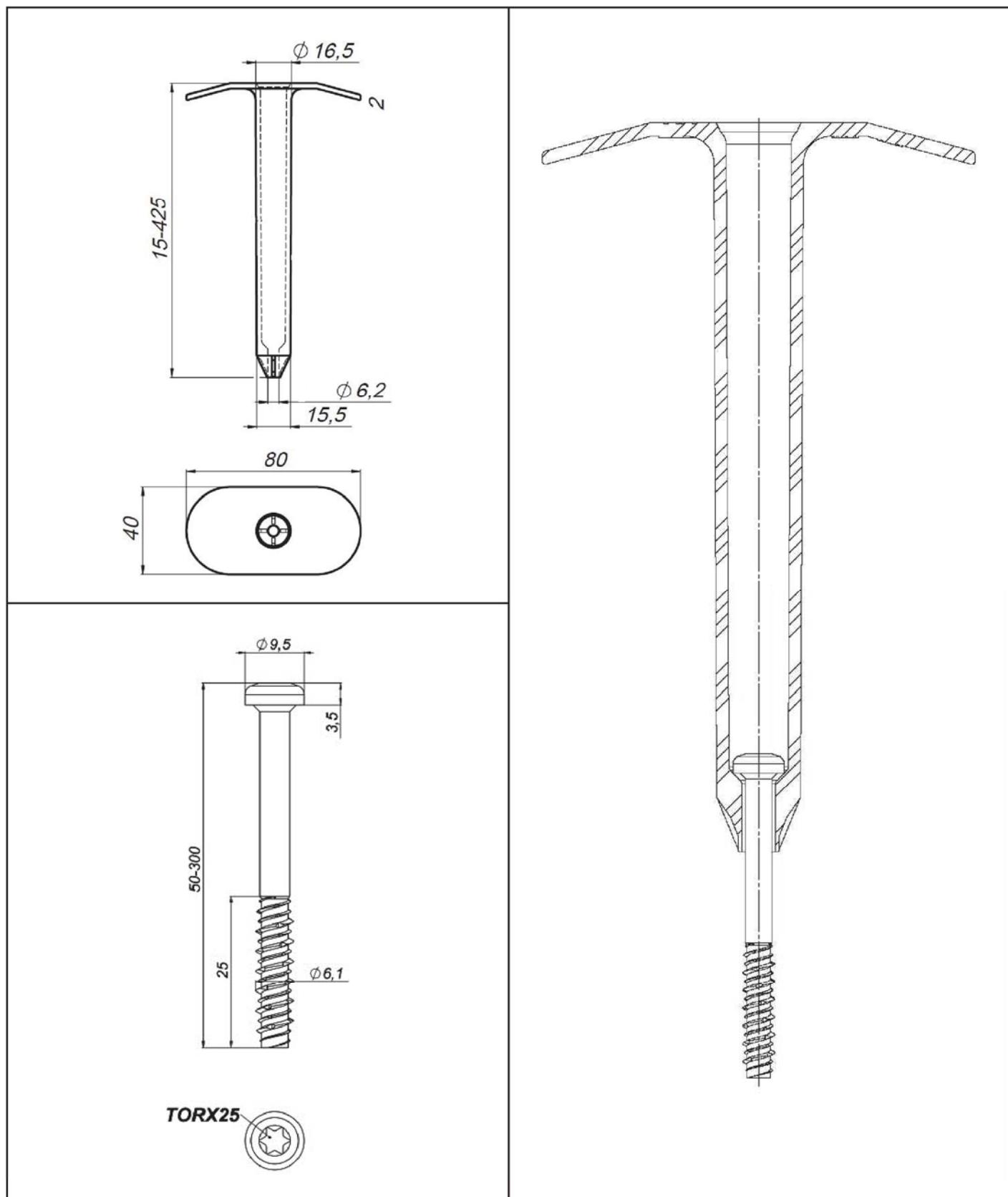
KOELNER S.A. Flat Roof Fasteners
