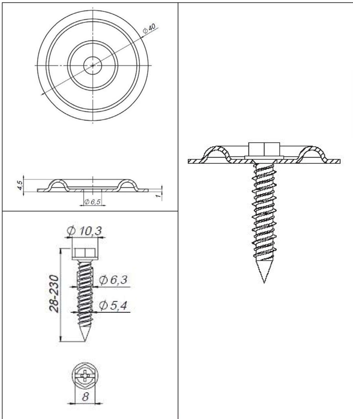
**KOELNER S.A. Flat Roof Fasteners**
