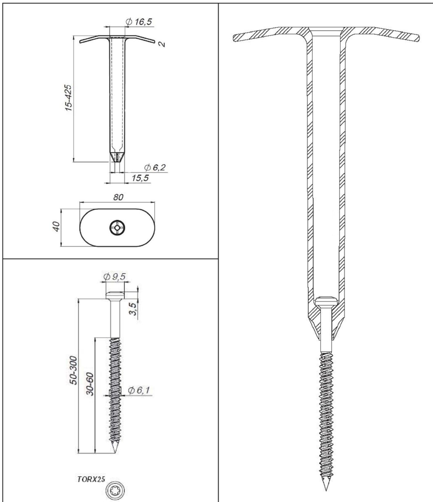
**KOELNER S.A. Flat Roof Fasteners**
