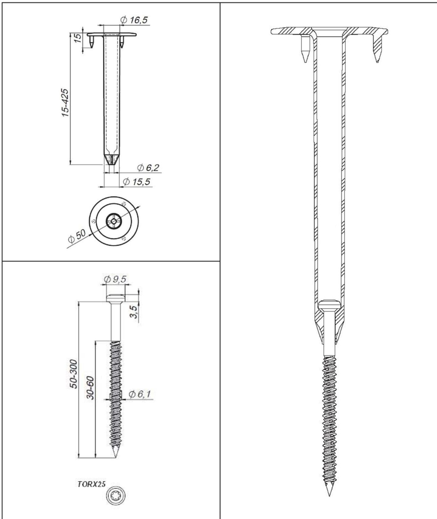
**KOELNER S.A. Flat Roof Fasteners**
