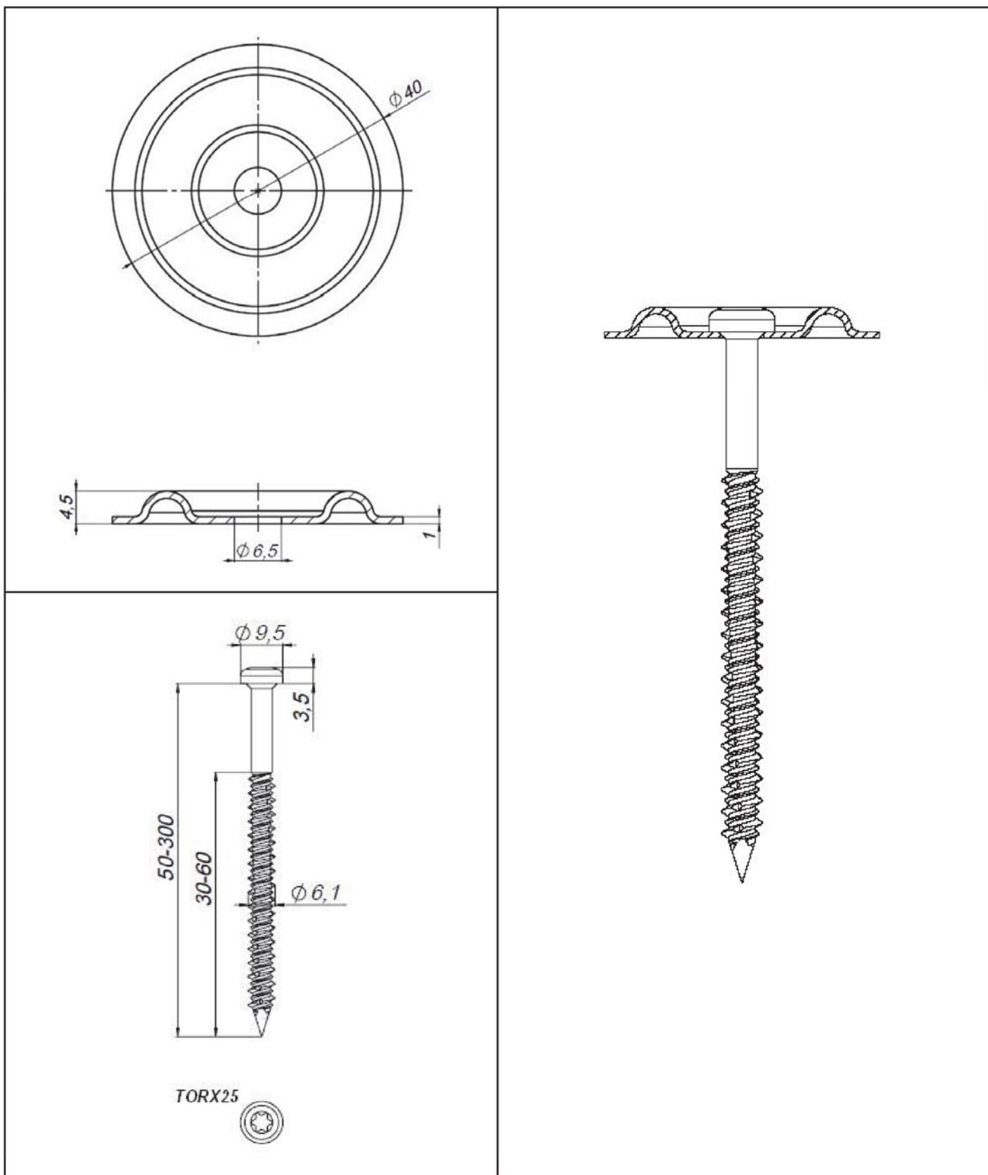
**KOELNER S.A. Flat Roof Fasteners**
