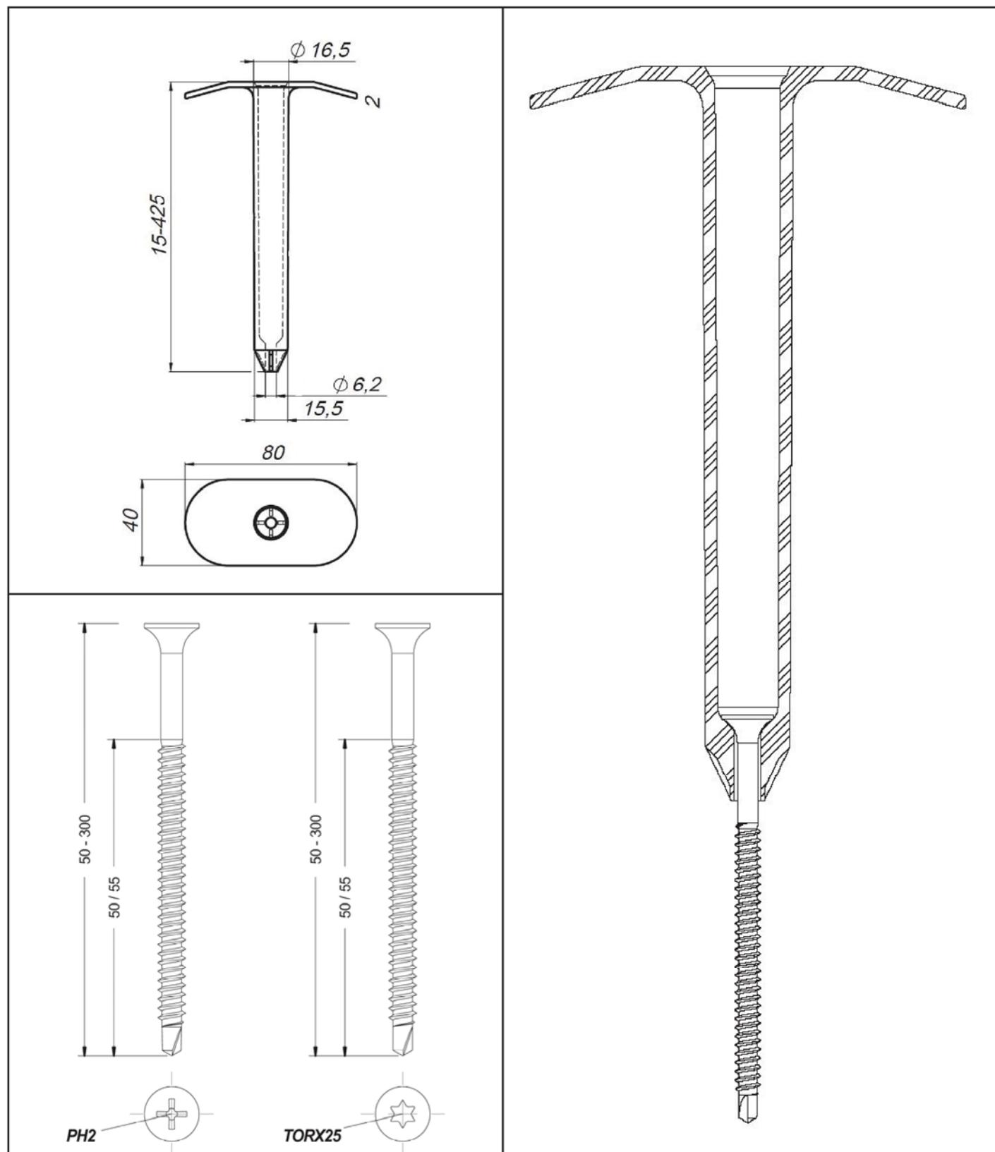
**KOELNER S.A. Flat Roof Fasteners**
