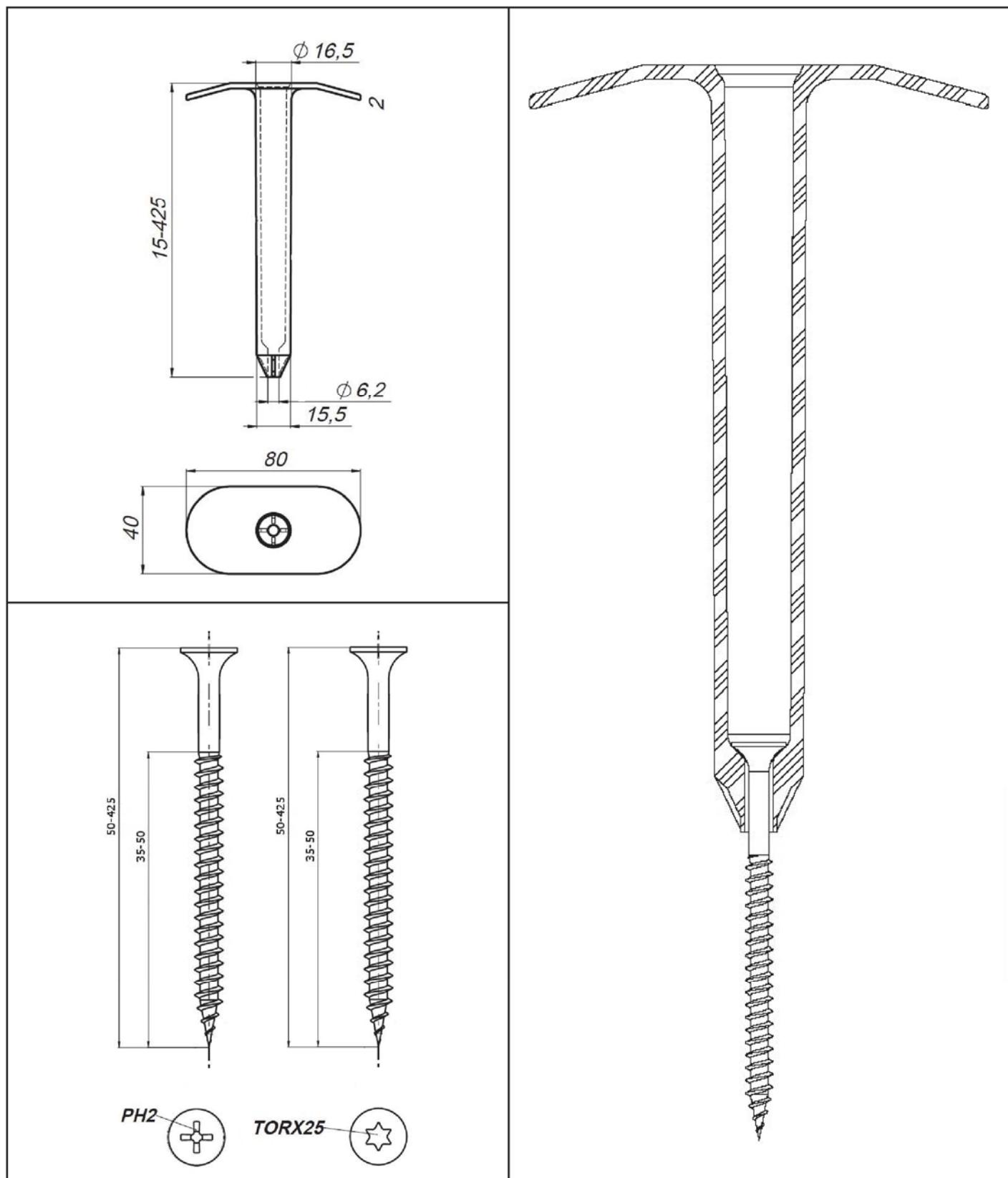
**KOELNER S.A. Flat Roof Fasteners**
