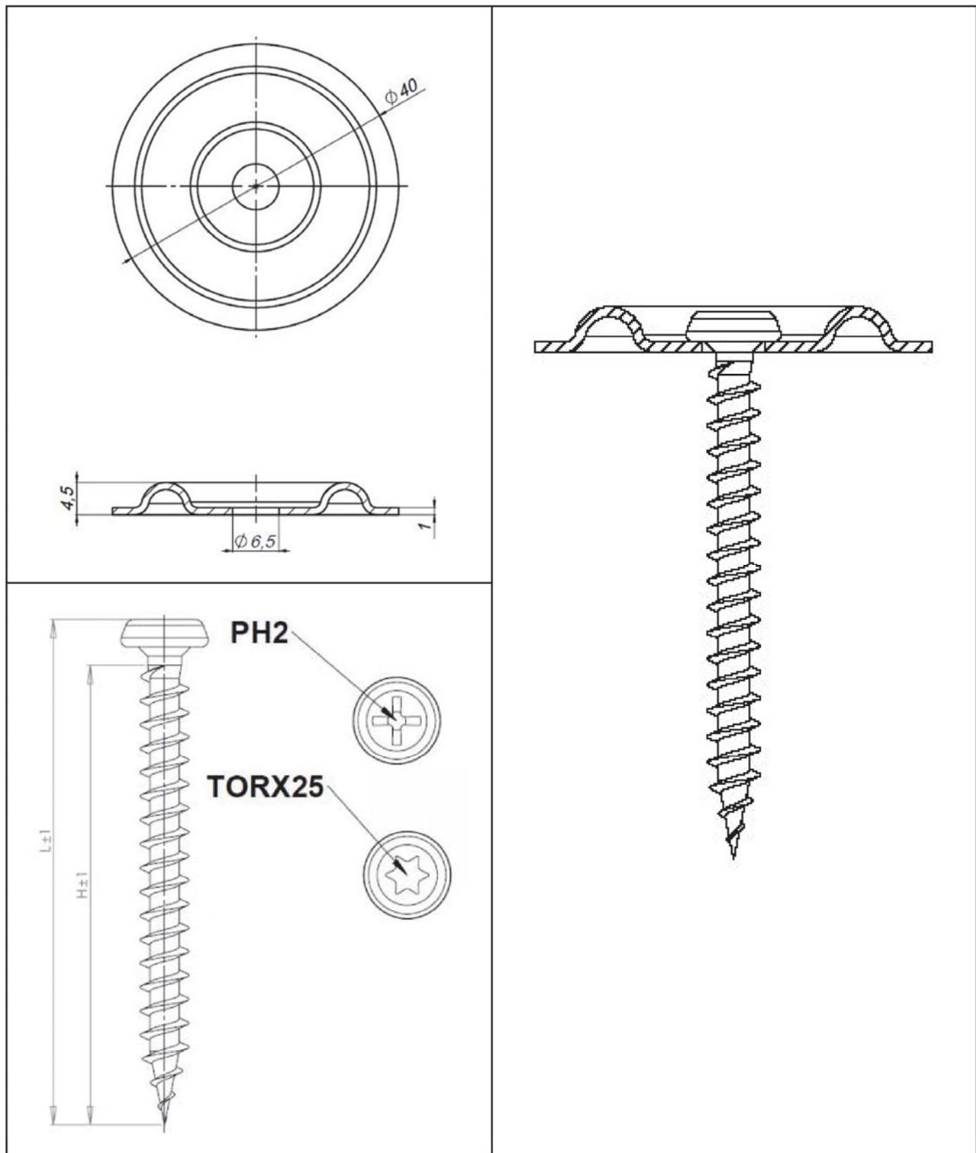
**KOELNER S.A. Flat Roof Fasteners**
