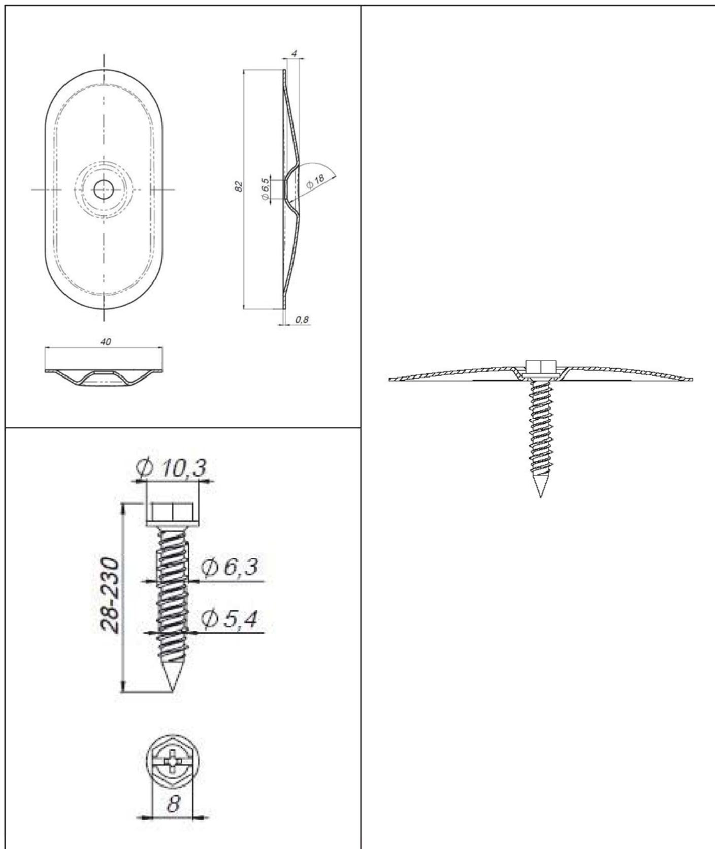
**KOELNER S.A. Flat Roof Fasteners**
