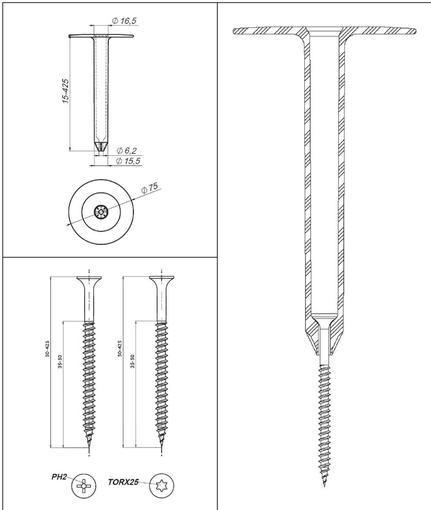
**KOELNER S.A. Flat Roof Fasteners**
