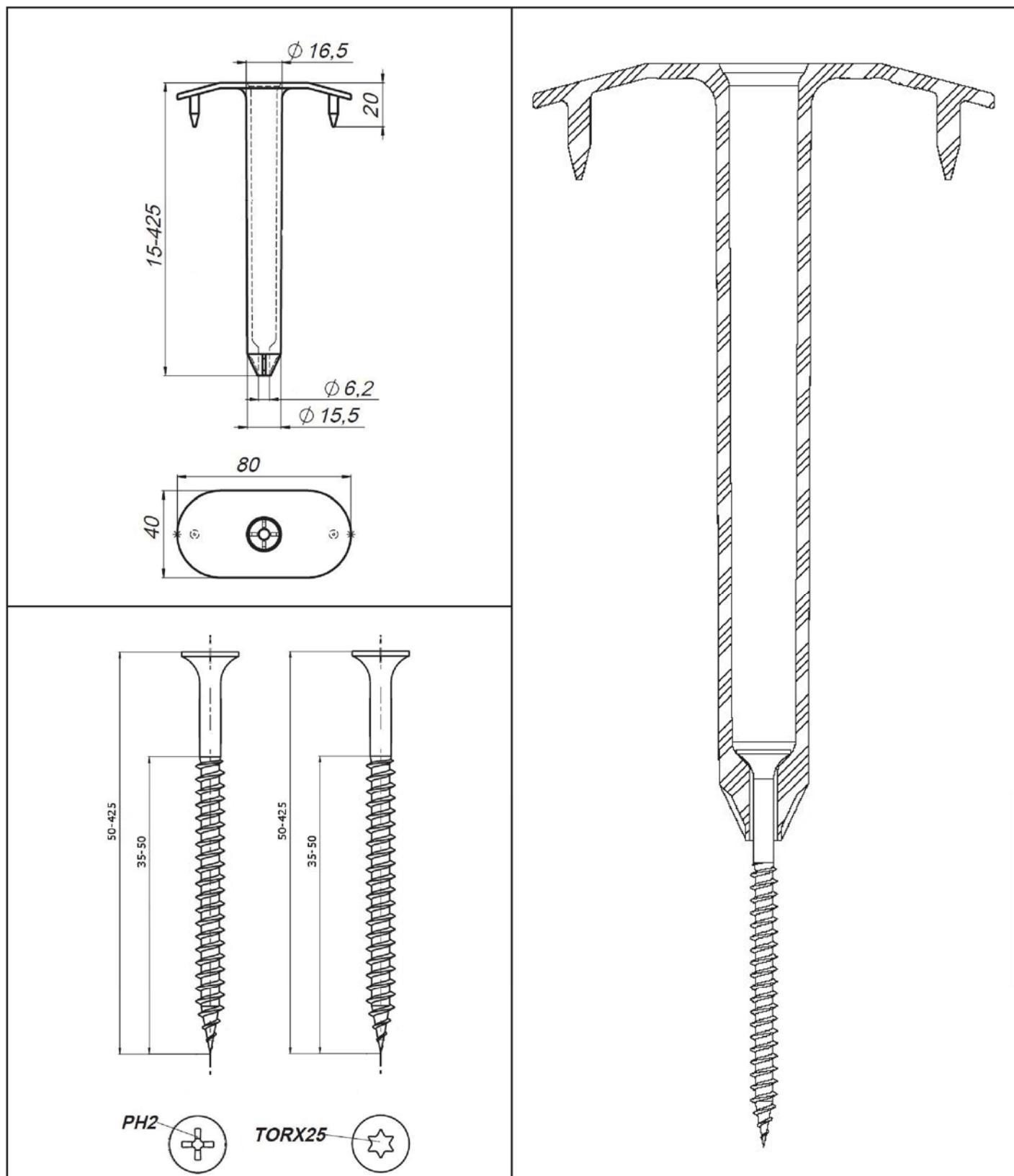
**KOELNER S.A. Flat Roof Fasteners**
