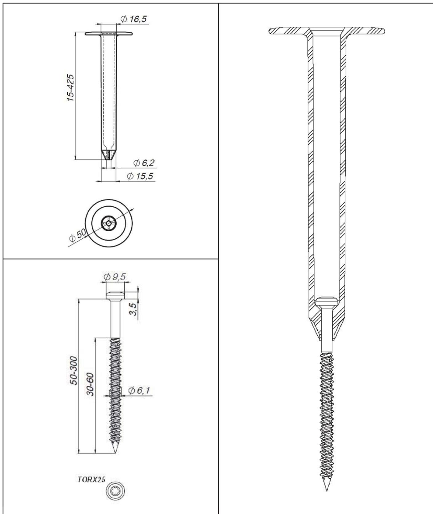
**KOELNER S.A. Flat Roof Fasteners**
