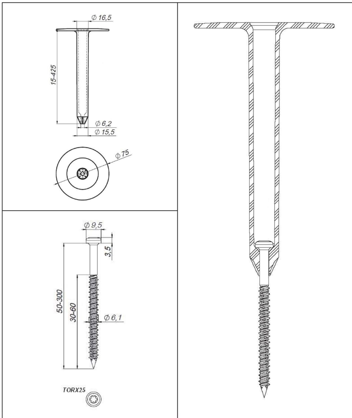
**KOELNER S.A. Flat Roof Fasteners**
