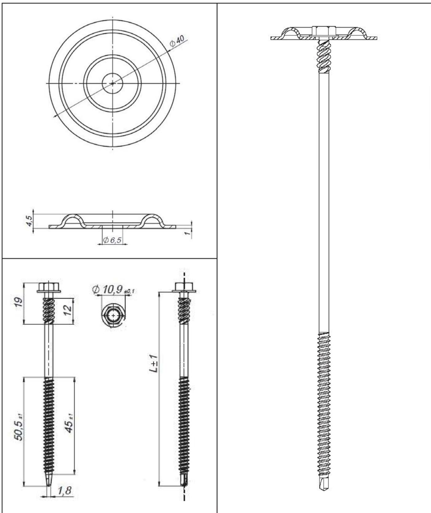
**KOELNER S.A. Flat Roof Fasteners**
