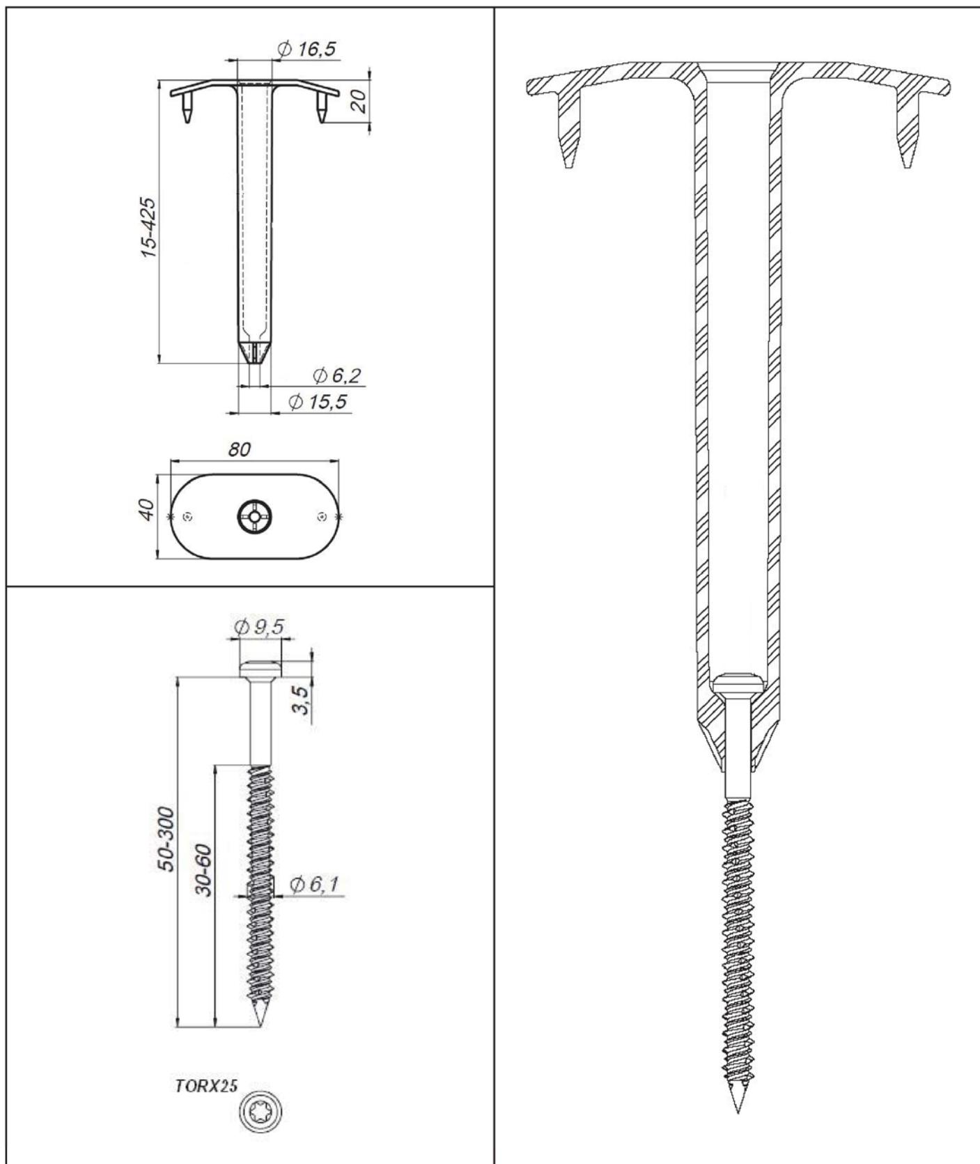
**KOELNER S.A. Flat Roof Fasteners**
