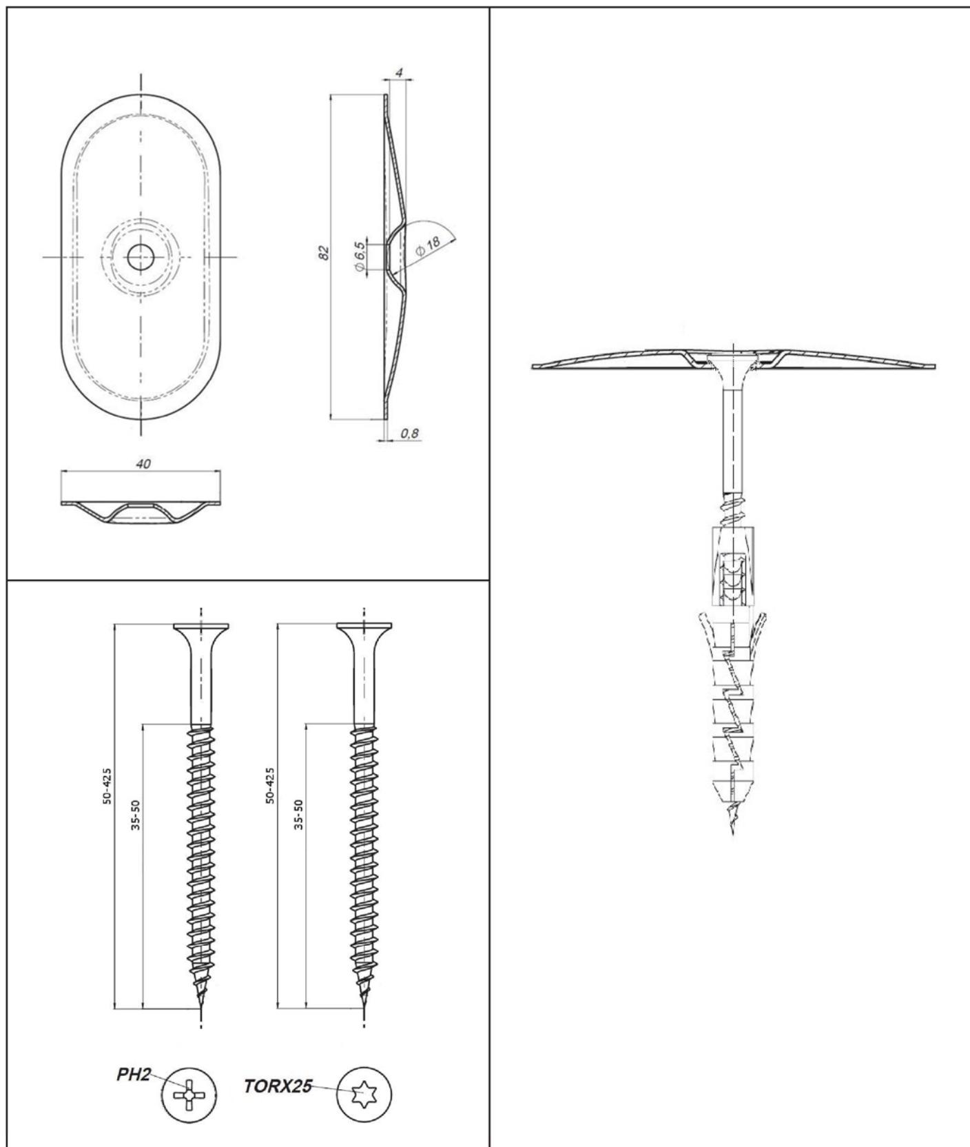
**KOELNER S.A. Flat Roof Fasteners**
