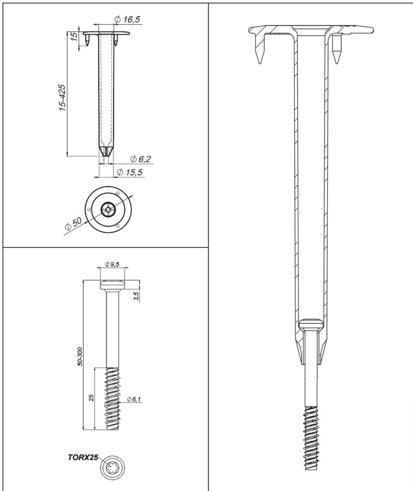
KOELNER S.A. Flat Roof Fasteners
