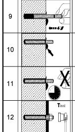
Push the threaded rod or reinforcing bar into the anchor hole while turning slightly to ensure positive distribution of the adhesive until the embedment depth is reached.
