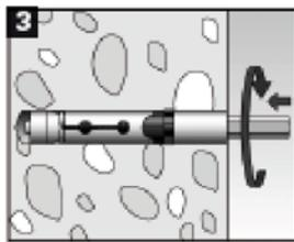
3.) Tightening the anchor. Tightening with the included hexagon in the package is preferred. Other tightening methods are allowed.
