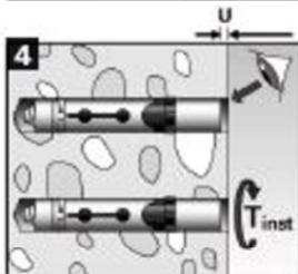
4.) Tighten the anchor into the concrete until the gap  $U$  is 3-5 mm or the installation torque is reached. Only one requirement has to be fulfilled.
