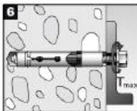
6.) Tightening the anchor with the torque  $\leq T_{max}$ .
