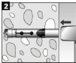
2.) Hammering in the anchor flushed with the surface of the concrete.
