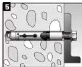
5.) Connecting the fixing and the anchor with a fitting fastener. The length of the fastener should be determined depending on the thickness of fixture  $t_{fix}$ , admissible tolerances, and available thread length  $l_{s,max}$  and  $l_{s,min}$  including the gap  $U$ .
