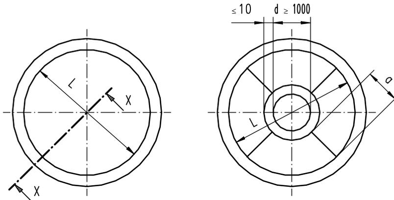
Figure B.3 - Subdivision of recessed SMF sheets for spherical sliding surfaces
