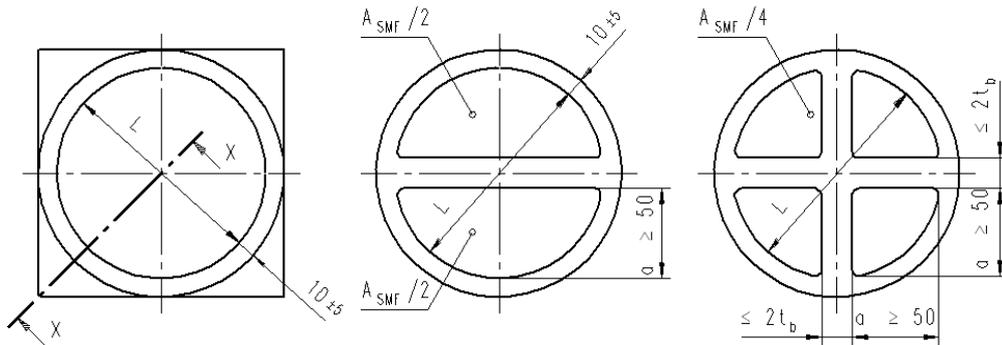
Figure B.2 - Examples of recessed flat SMF configurations
