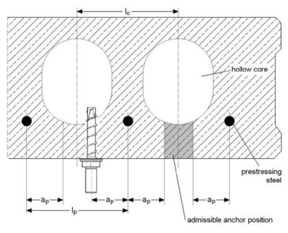
$\begin{array}{lll} \text{core distance} & & I_c & \geq 100 \text{ mm} \\ \\ \text{prestressing steel} & & I_p & \geq 100 \text{ mm} \\ \\ \text{distance} & & \\ \\ \text{distance between anchor} & & \\ \text{ap} & \geq 50 \text{ mm} \\ \\ \text{steel} & & \\ \end{array}$
