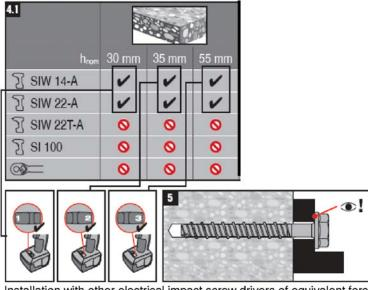
Hand setting of HUS-HR in concrete base material not allowed (machine setting only).
