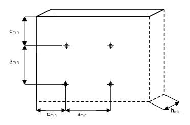
Additional installation data for precast prestressed hollow core slabs and minimum member thickness, spacing and edge distance
