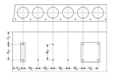
Minimum edge distance  $c_{min}$  ≥ 100 mm
