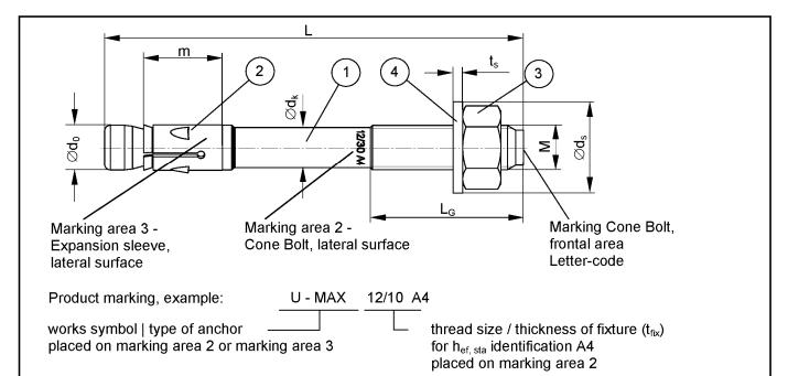
Letter-code on the frontal area of the cone bolt and maximum thickness of fixture  $t_{\text{fix}}$ :
