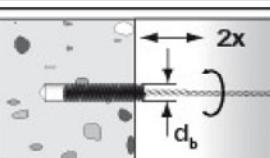
Brush the drill hole two times. For drill hole  $\geq 30\text{ mm}$  use a power drill.
