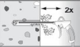
Clean the drill hole: Blow out the drill hole two times, using oil-free compressed air ( $P > 6\text{bar}$ )
