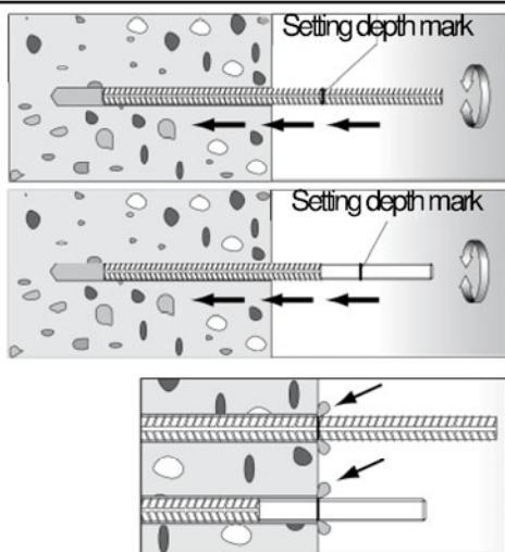
Only use clean and oil-free rebars. Mark the setting depth of the reinforcing bar. Using a turning movement, push the reinforcement bar or the FRA vigorously into the filled hole up to the insertion depth marking.
