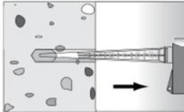
Fill approx. 2/3 of the drill hole with mortar. Always begin from the bottom of the hole and avoid bubbles.
