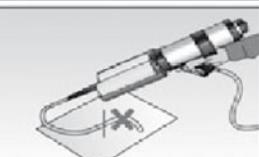
Press approx. 10 cm of material out until the resin is evenly grey in colour. Don't use mortar that is not uniformly grey.
