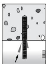
For overhead installations support the anchor rod with wedges.
