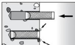
Only use clean and oil-free anchor elements. Mark the setting depth of the anchor. Press the anchor rod or internal threaded anchor down to the bottom of the hole, turning it slightly while doing so. After inserting the anchor element, excess mortar must emerge from the mouth of the drill hole.
