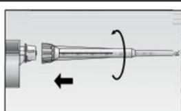
Twist on the static mixer (the spiral in the static mixer must be clearly visible).
