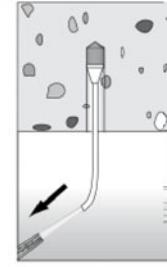
For overhead installation, deep holes  $h_0 > 250$  mm or drill hole diameter  $d_0 \geq 40$  mm use an injection-adapter.
