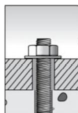
For in-place anchorage fill the annual clearance with mortar.
