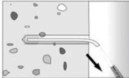
For drill hole depth  $\geq 150$  mm use an extension hose.
