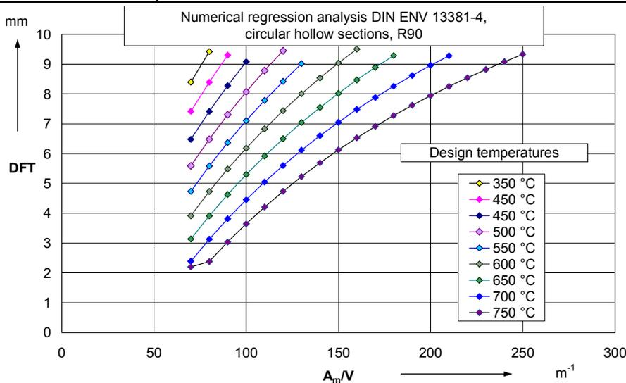
Annex 1, Table 25: Beams and columns, circular hollow sections
