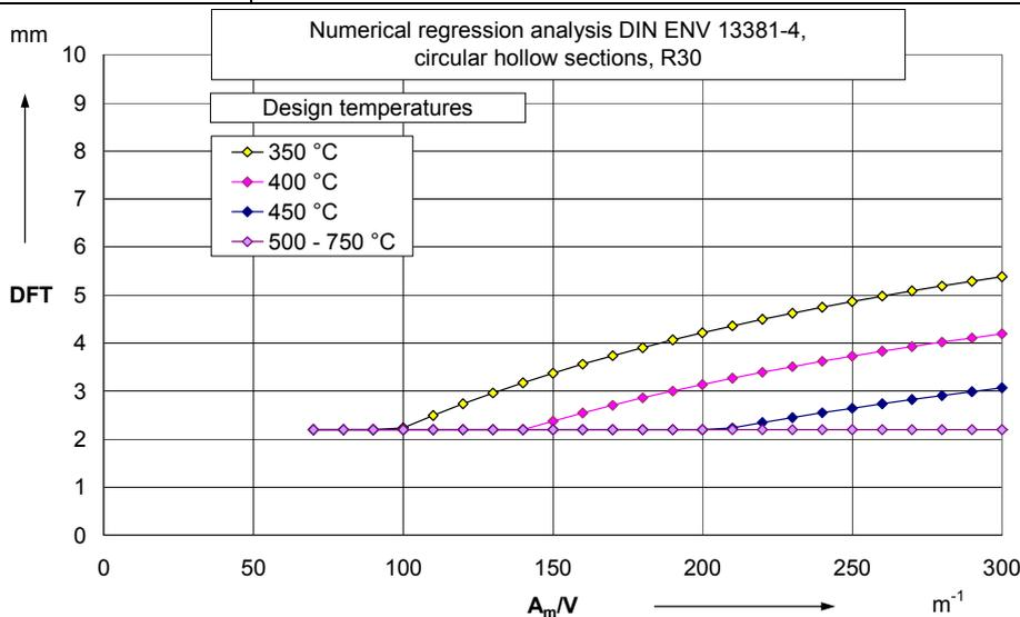
Annex 1, Table 22: Beams and columns, circular hollow sections
