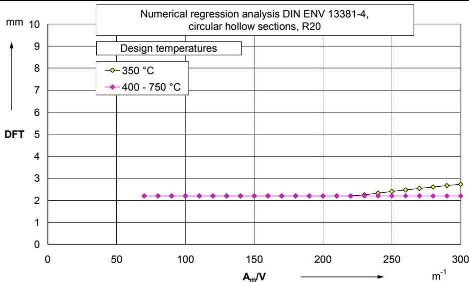
Annex 1, Table 21: Beams and columns, circular hollow sections
