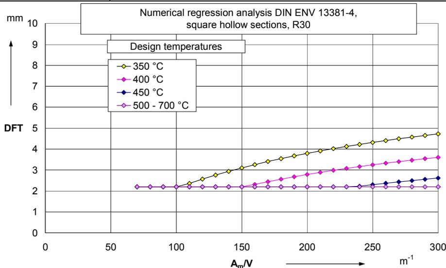
Annex 1, Table 15: Beams and columns, rectangular hollow sections
