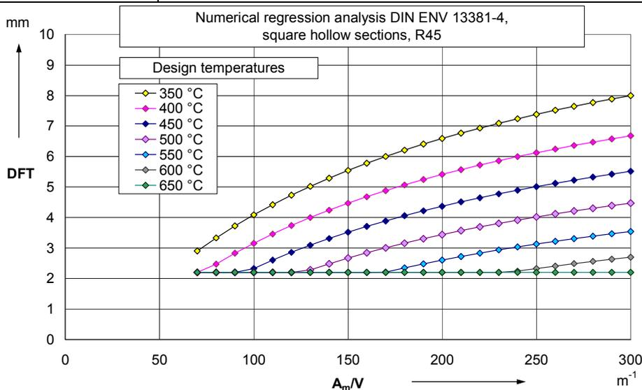
Annex 1, Table 16: Beams and columns, rectangular hollow sections
