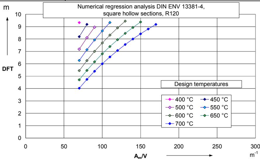
Annex 1, Table 19: Beams and columns, rectangular hollow sections
