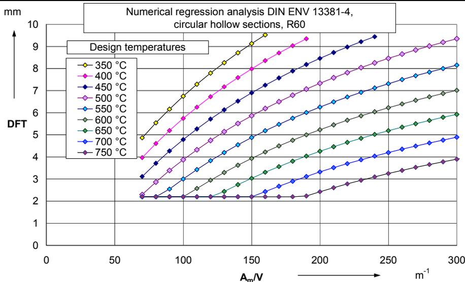
Annex 1, Table 24: Beams and columns, circular hollow sections
