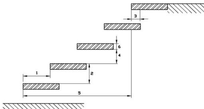
**Cantilever step stair system HGM**
