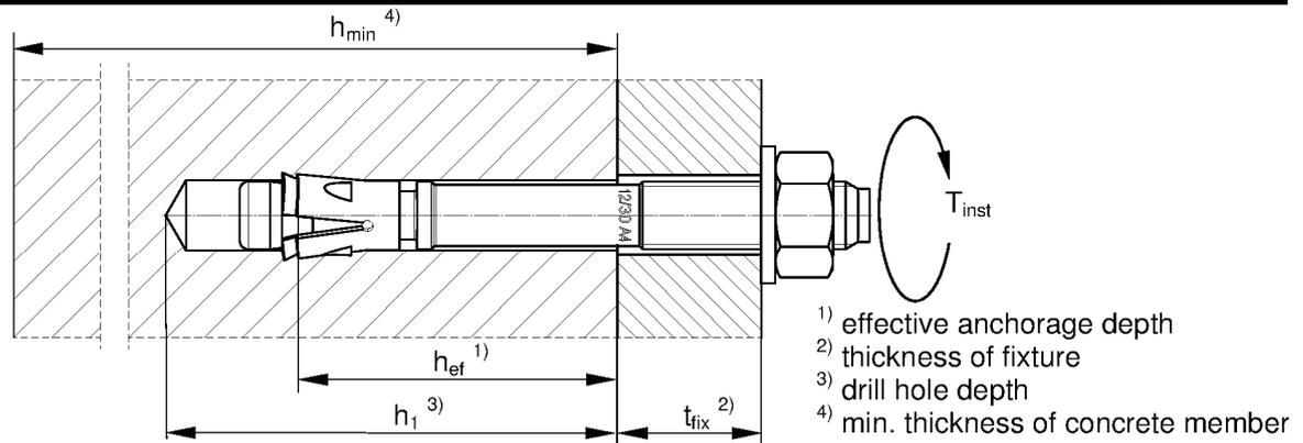
**Table 4: Minimum thickness of concrete members, minimum spacing and minimum edge distances of anchors**
