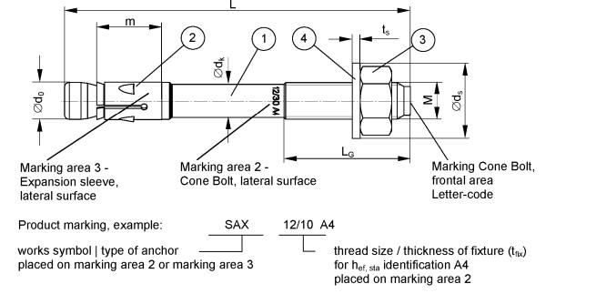
Letter-code on the frontal area of the cone bolt and maximum thickness of fixture  $t_{\text{fix}}$ :
