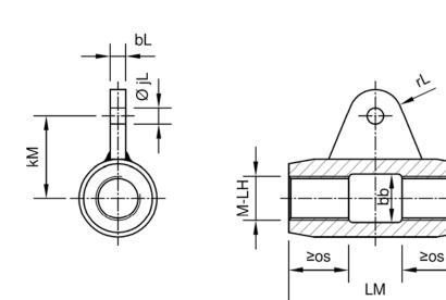
Minimum thread engagement of the tension rod = om - oj according to annex 3
