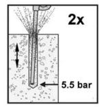
Blow 2 times with oil-free compressed air (min. 5.5 bar) and verify that the threaded rod and rebar can achieve the required embedment depth.
