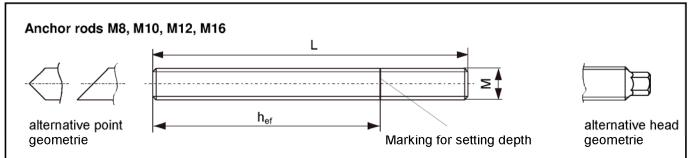
**Table 1:** Installation parameters anchor rods in solid bricks (without perforated sleeves)
