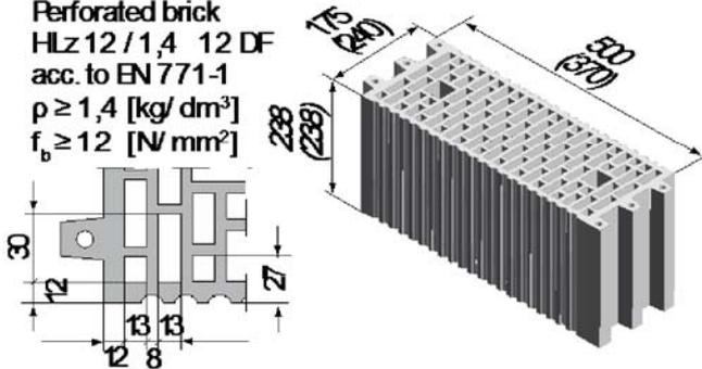
**Brick No. 2** Perforated brick acc. to EN 771-1
