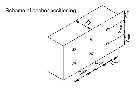
Minimum spacing and edge distances Minimum thickness of member
