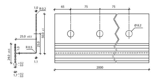
**Vertical connection profile – "SCHWEPA Verbindungsleiste Alu"** (dimensions in mm) length: 590 mm
