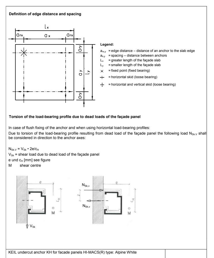
Definition of edge distance and spacing Torsion of load-bearing profile
