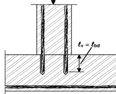
**Figure 5:** Anchoring of reinforcement to cover the line of acting tensile force
