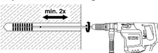
For boreholes deeper than 250mm (for  $d_s=8\text{mm}-12\text{mm}$ ) resp. deeper than  $20x d_s$  (for  $d_s > 12\text{mm}$ ) use machine brushing and brush extensions HIT-RBS (see table 6 and 7).
