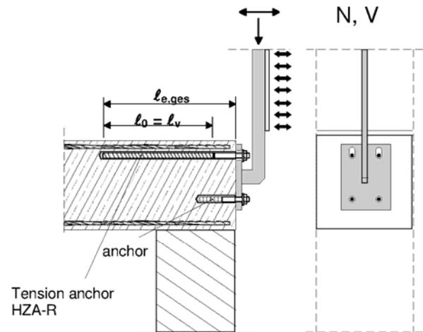
**Figure 8:** Overlap joint for the anchorage of cantilever members
