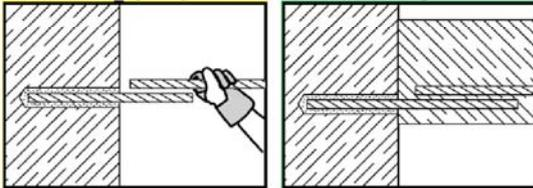
Load may be applied only after the curing time " $t_{cure}$ " has elapsed. See table below.
