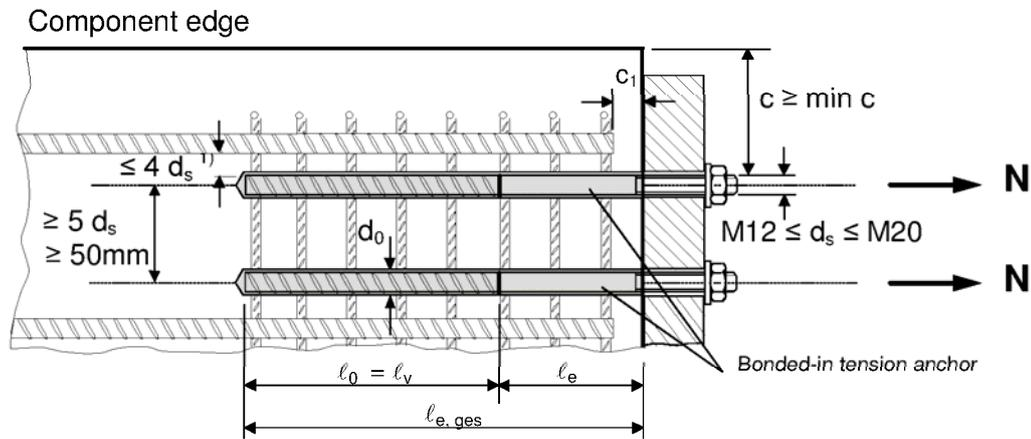
1) If the clear distance between spliced bars exceeds  $4d_s$ , then the lap length shall be increased by the difference between the clear bar distance and  $4d_s$ .
