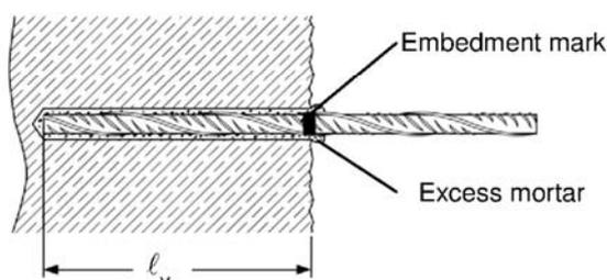
After installing the rebar the annular gap must be completely filled with mortar.
