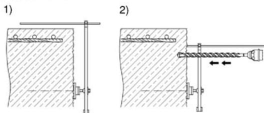
For holes  $l_b > 20$  cm use drilling aid. Three different options can be considered:
