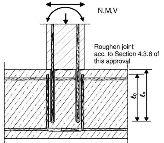
**Figure 3:** End anchoring of slabs or beams, designed as simply supported
