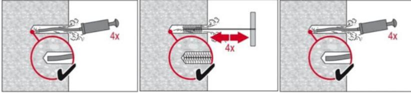
As an alternative to compressed air cleaning, a manual cleaning is permitted for hammer drilled boreholes up to hole diameters  $d_0 \leq 20\text{mm}$  and depths  $l_v$  resp.  $l_{e,ges.} \leq 160\text{mm}$  or  $10 * d$ .
