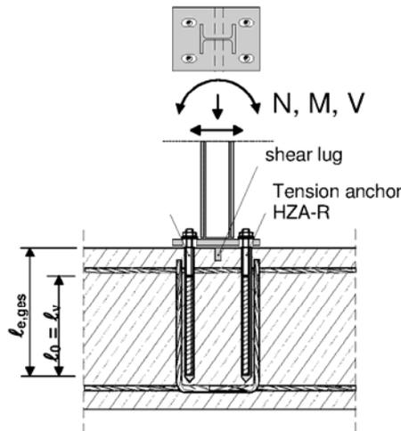
**Figure 7:** Overlap joint for the anchorage of barrier posts
