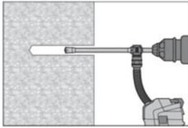
Drill hole to the required embedment depth with an appropriately sized Hilti TE-CD or TE-YD hollow drill bit with Hilti vacuum attachment. This drilling system removes the dust and cleans the bore hole during drilling when used in accordance with the user's manual.
