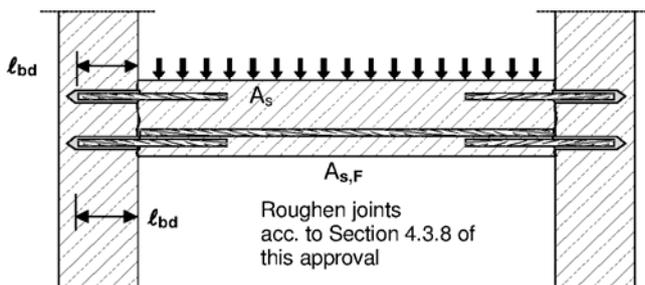
**Figure 4:** Rebar connection for components stressed primarily in compression. The rebars are stressed in compression.
