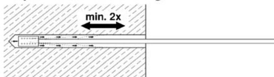
For boreholes deeper than 250mm (for  $d_s=8\text{mm}-12\text{mm}$ ) resp. deeper than  $20x d_s$  (for  $d_s > 12\text{mm}$ ) use the appropriate air nozzle Hilti HIT-DL (see table 6 and 7).
