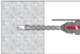
Or drill hole to the required embedment depth using a hammer-drill with carbide drill bit set in rotation hammer mode, a compressed air drill or a diamond coring machine.
