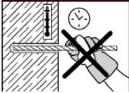
Observe the working time " $t_{work}$ ", which varies according to temperature of base material. Minor adjustments to the rebar position may be performed during the working time. See table below.
