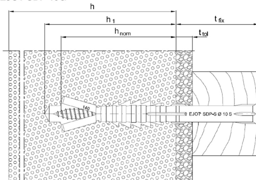
**Picture 1: Intended use: screw head-type: countersunk (S)**
