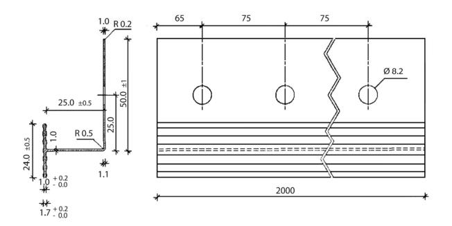
**Vertical connection profile – "INTRATHERM Verbindungsleiste Alu"** (dimensions in mm) length 590 mm
