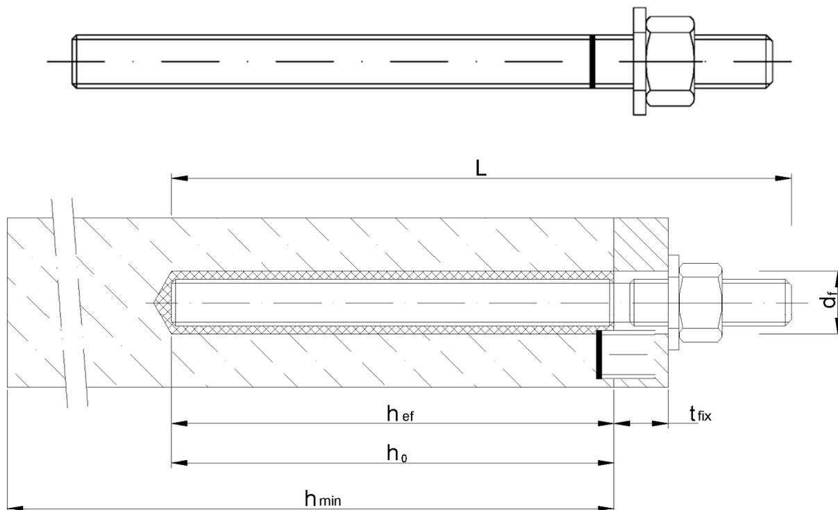
**REINFORCING BAR  $\varnothing 8, \varnothing 10, \varnothing 12, \varnothing 14, \varnothing 16, \varnothing 20, \varnothing 25, \varnothing 28, \varnothing 32$  (acc. to Annex 4)**
