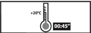
9. Allow the adhesive to cure to the specified time prior to applying any load or torque. Do not move or load the anchor until it is fully cured (attend Table 4).
