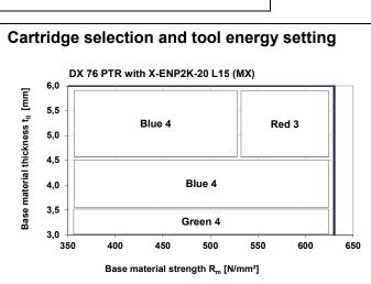
Job-site trials are recommended to prove proper energy setting. If required, fine adjustment of energy setting.
