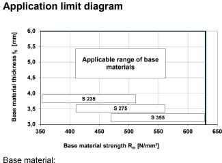
Structural steel S235, S275 and S355 in qualities JR, JO, J2, K2 according to EN 10025-2; minimum nominal thickness = 3 mm, specific details on minimum thickness see Annex 6
