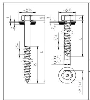
Fastener: stainless steel (1.4301) – EN 10088 Washer: stainless steel (1.4301) – EN 10088
