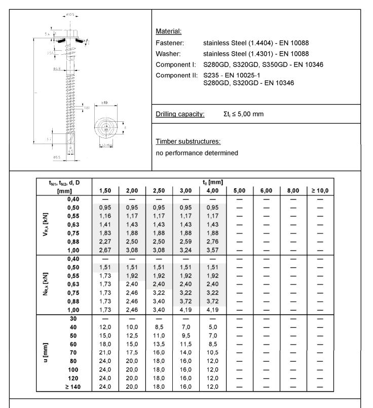
If component  $t_{N1}$  resp.  $t_{N2}$  is made of S320GD or S350GD the grey highlighted values may be increased by 8%.
