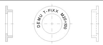
Data clip: section, top view (with example for marking) and side view
