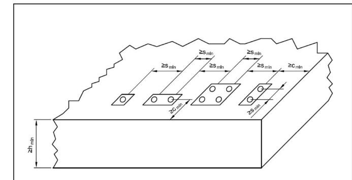
The mentioned spacings, edge distances and member thicknesses apply also for fixing anchors installed in the front edge.
