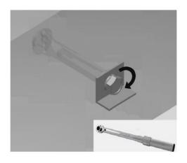
Apply torque moment with the help of a torque wrench.  $T_{\text{inst}}$  must not be exceeded.
