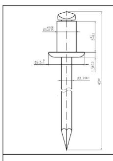
Sleeve: Aluminum AlMg3 – EN 573 Mandrel: Steel galvanised – EN 10016-2
