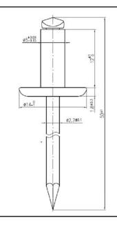
Sleeve: Aluminum AlMg3 – EN 573 Mandrel: Steel galvanised – EN 10016-2
