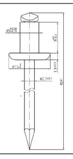
Sleeve: Aluminum AlMg3 – EN 573 Mandrel: Steel galvanised – EN 10016-2
