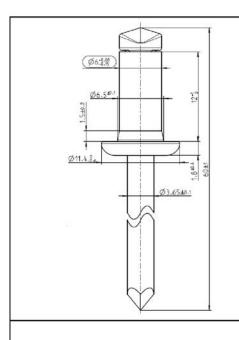
Sleeve: Steel galvanised – EN 10016-2 Mandrel: Steel galvanised – EN 10016-2
