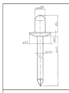
Sleeve: Aluminum AlMg5 – EN 573 Mandrel: Steel galvanised – EN 10016-2
