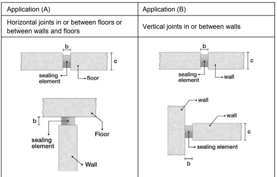
For the choice of the sealing element ("Litaflex-Faltelement" or "Litaflex-Fugenblock") and the thickness and width of the sealing element, see Table 2.0 and 2.1 and the manufacturer's instructions.
